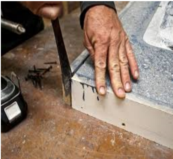
Fig3.1 Remove the mold
