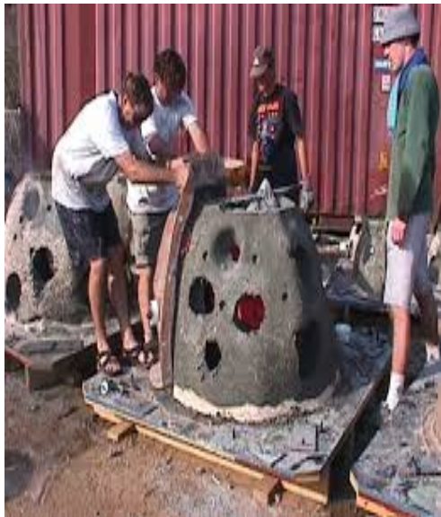
Fig3.1 Remove the mold
