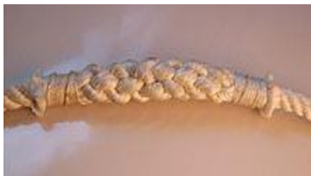
Short splice, with ends whipped
