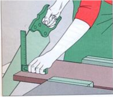
Checking a saw with a try square
