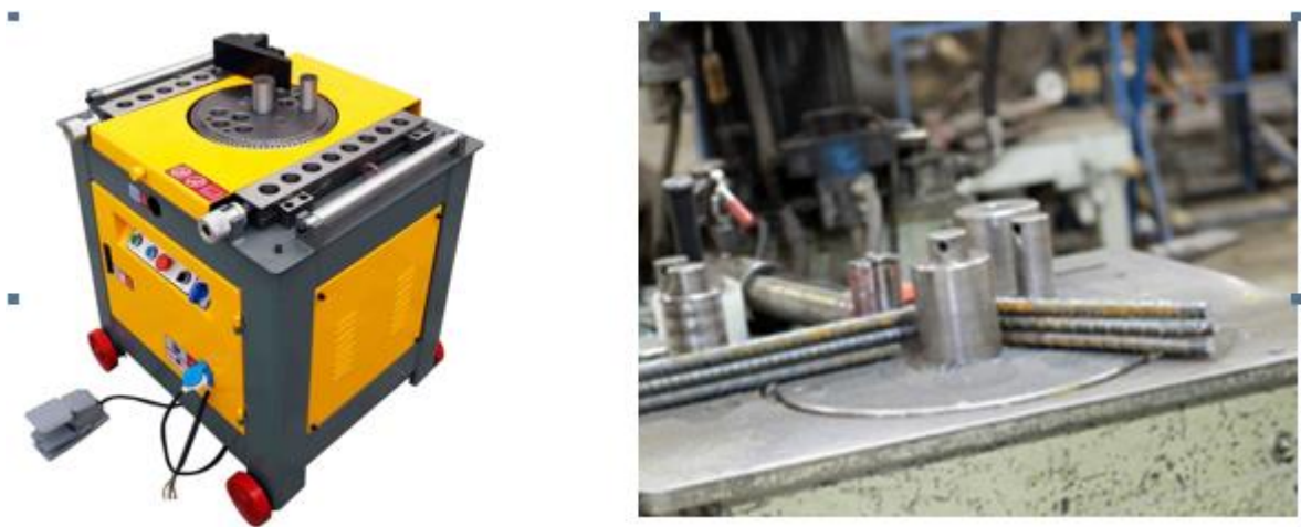
Fig.3 Example of bar bending machine
