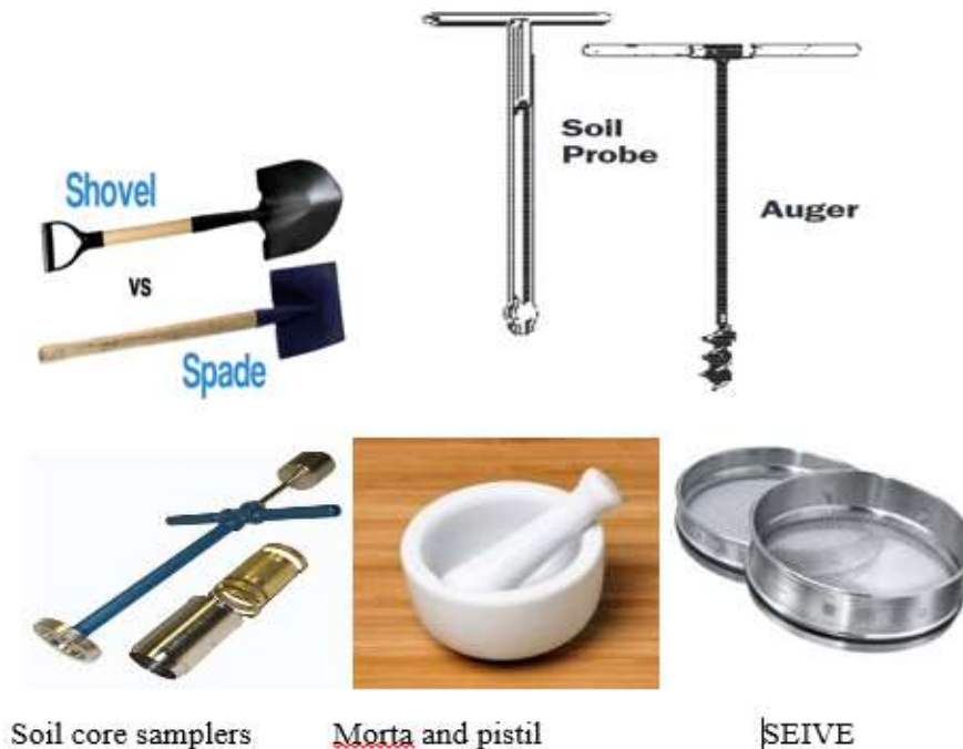
Fig.1.1. Tools for Soil Sampling
