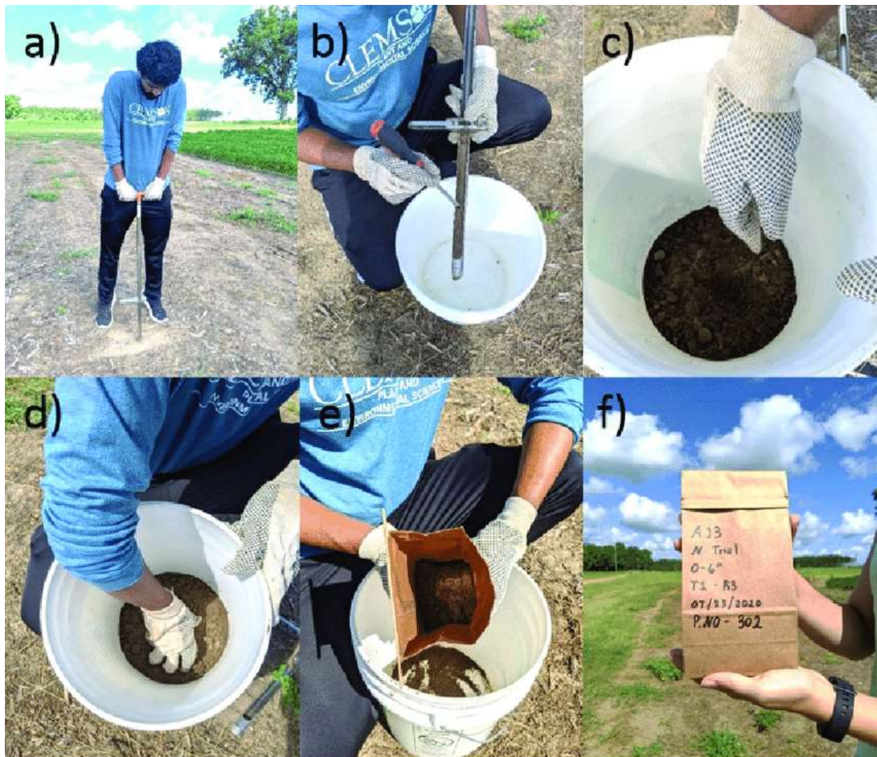
Fig 2.5. Soil sampling to labeling steps
