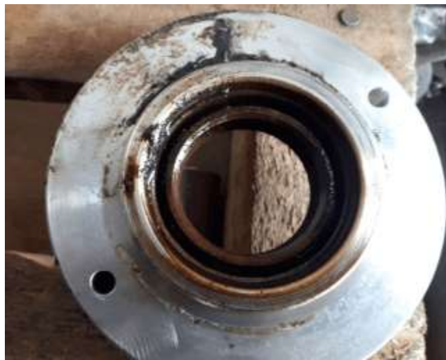
Fig.4.2: Seal leak causing bearing contamination and subsequent failure
