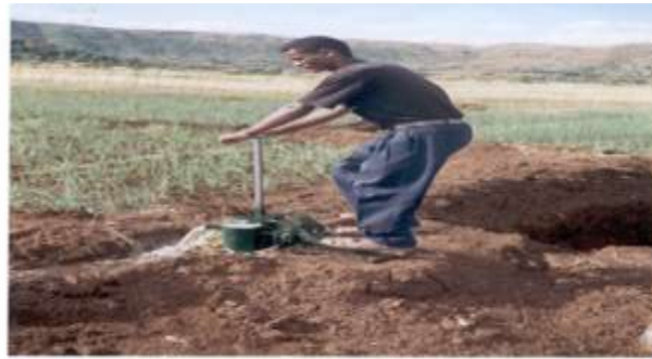
Fig.2.10: Typical treadle irrigation pump
