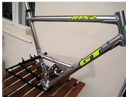
Figure 43: Welded aluminium alloy bicycle frame
