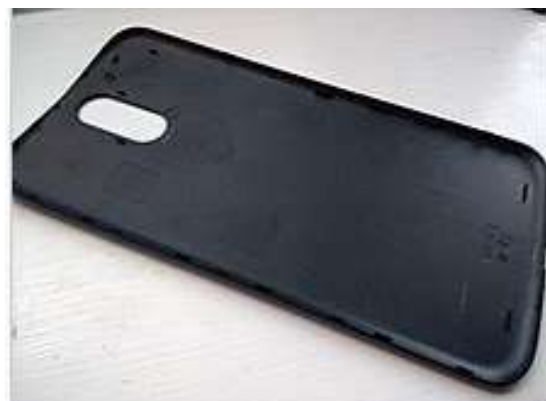
Figure 44: Cell phone frame made from Polycarbonate
