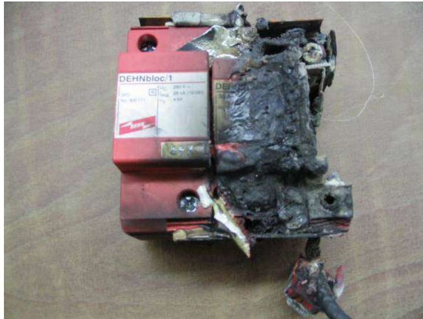
Image 3: Short circuit and overvoltage converter
