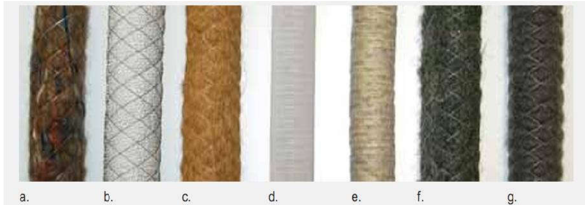
Figure_2.3: Envelopes can be made of wrapped polypropylene fibers (a, f & g), polystyrene granules (b) and coconut fibers (c), non-woven nylon (d) and woven type (e)
