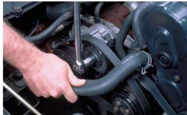
P4-5 Loosen the hold-down fastener for the tensioner or generator pulley.
