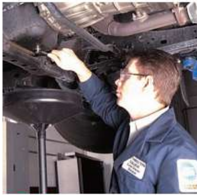
P3-11 Tighten the drain plug according to the manufacturer's recommendations. Overtightening can cause thread damage, whereas undertightening can cause an oil leak.
