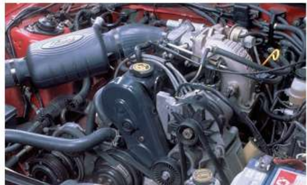
P4-15 Start the engine and check the belt for proper operation.
