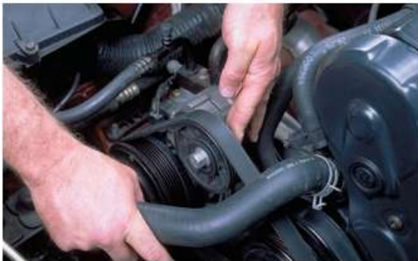
P4-4 To replace a worn belt, locate the tensioner or generator pulley.
