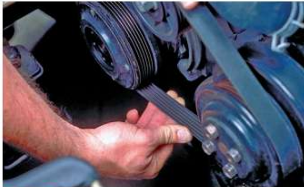
P4-12 Measure the belt deflection in its longest span. If a belt tension gauge is available, use it and compare the tension to specifications.
