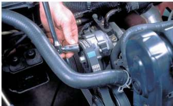
P4-14 Tighten the tensioner or generator pulley fastener.
