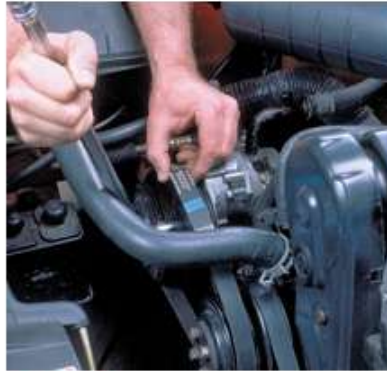
P4-10 Pry out the tensioner or generator pulley to put tension on the belt.
