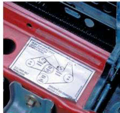
P4-8 Observe the belt routing diagram in the engine compartment.
