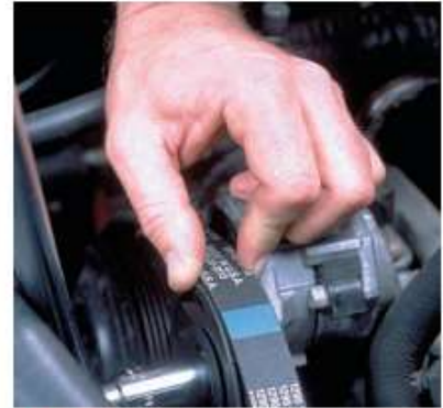
P4-11 Install the belt squarely in the grooves of each pulley.
