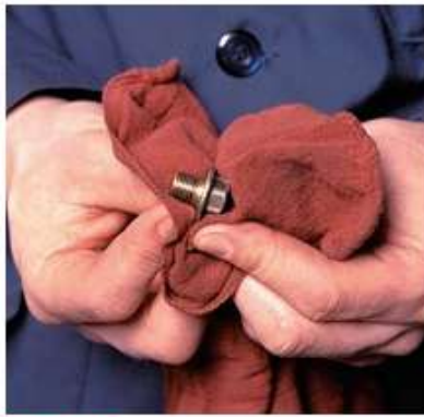
P3-10 Prior to installing the drain plug, wipe off its threads and sealing surface with a clean rag.
