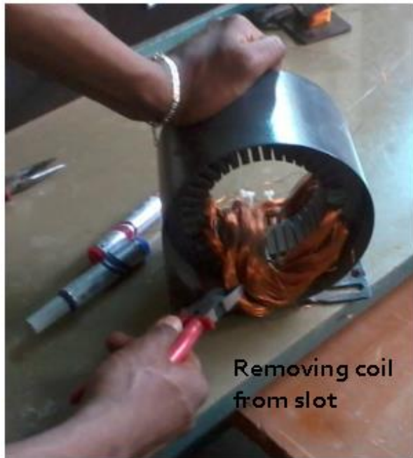
Figure 3.2 removing burn out coil
