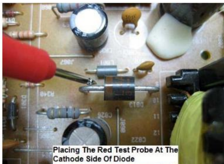
Figure2.102. Placing the RED test probe to the Secondary Output Diode Cathode Side.
