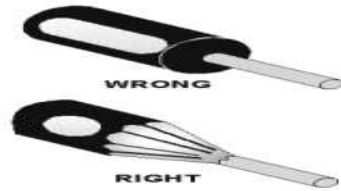
Figure1.2.2 Knife stripping.
