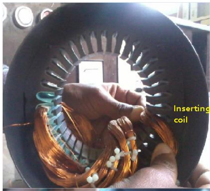
Figure 3.5 coil insertion
