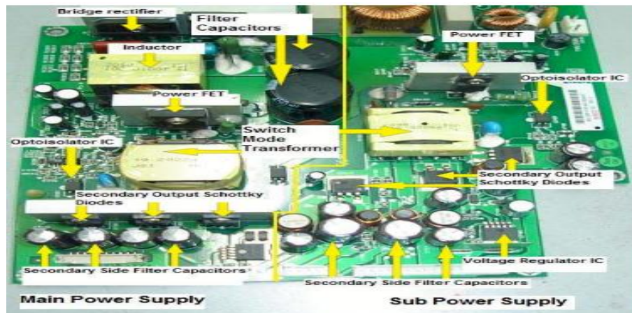
Figure2.33 typical LCD Monitor SMPS
