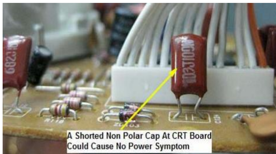
Figure2.105 Shorted Non Polar Capacitor at CRT Board.
