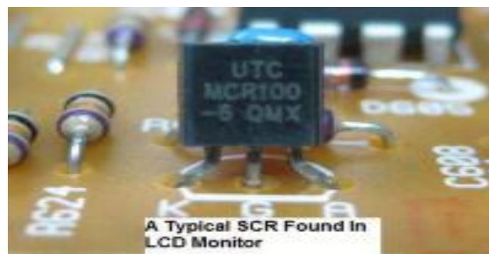
Figure2.70 Silcom Controlled Rectifier
