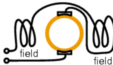
Figure.3. 43 Uncompensated series AC motor.
