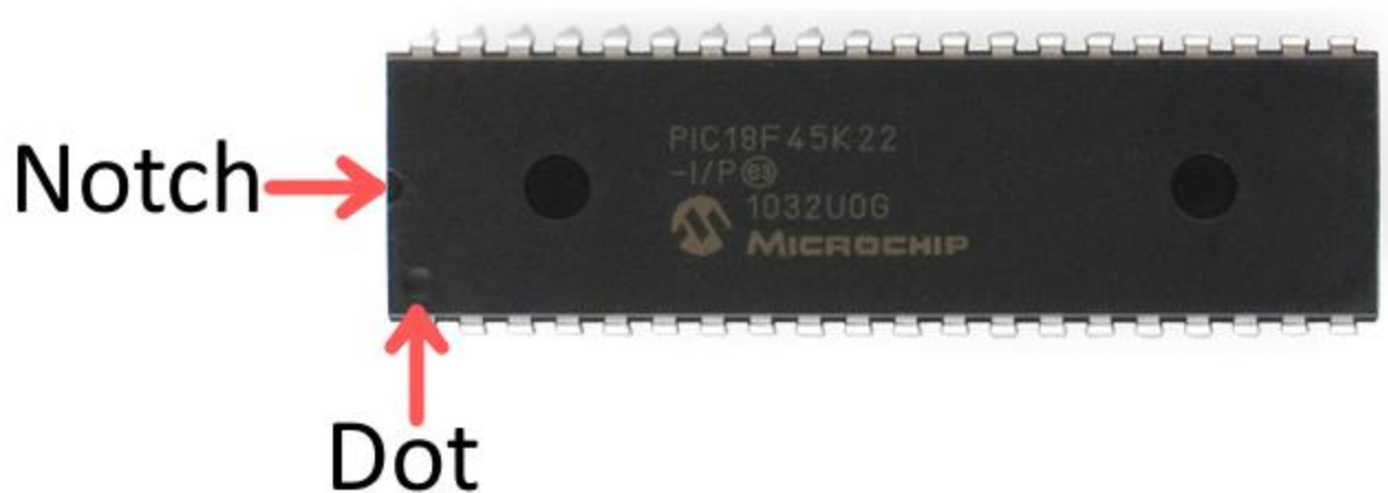
Figure 2.8: Polarity and pin numbering of ICs
