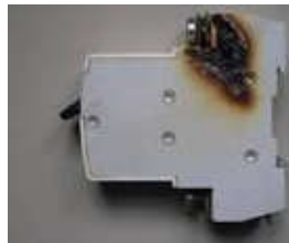
Figure 2. 1 circuit breaker defect
