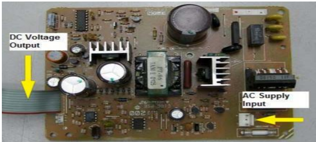
Figure2.32. A dot matrix Power Supply Board
