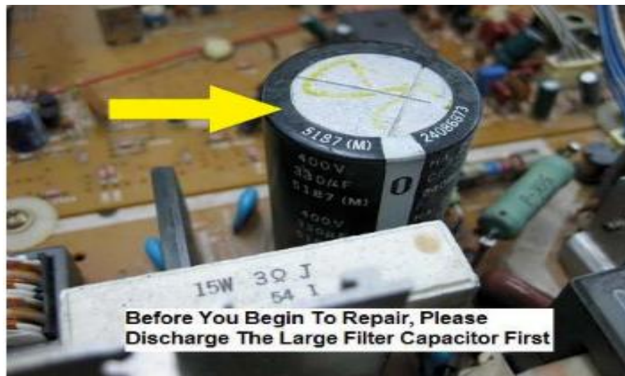
Figure3.9 Discharging the Big Capacitor
