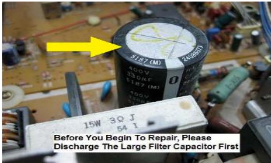
Figure3.9 Discharging the Big Capacitor
