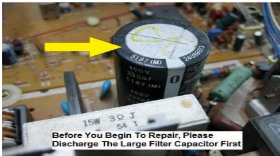
Figure3.10 Discharging the Big Capacitor with a 2.2Kohm 10watt resistor
