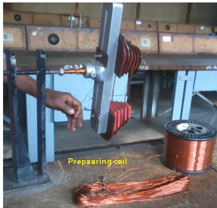
Figure 3.3 coil preparation
