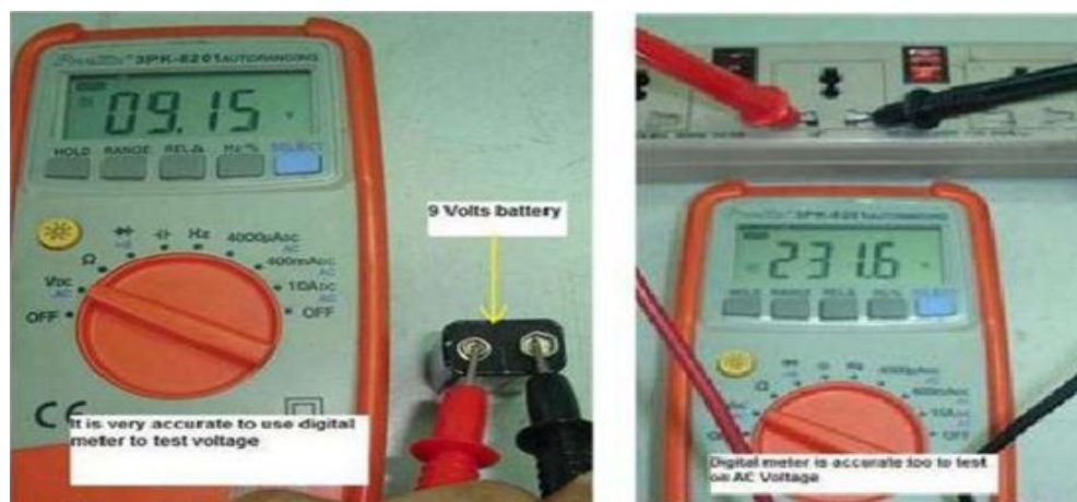
Figure 2.3 Measuring the voltage using digital meter.
