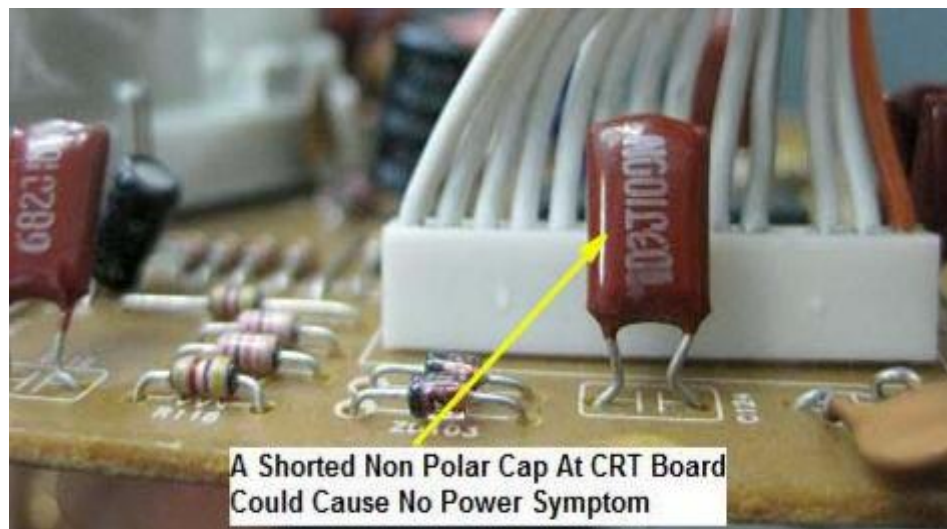
Figure2.105 Shorted Non Polar Capacitor at CRT Board.
