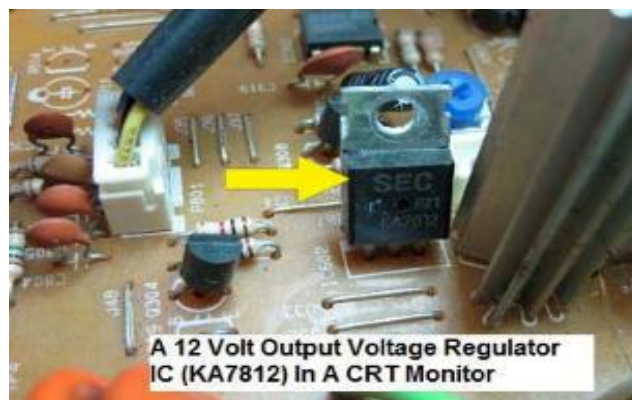
Figure2.80. Voltage Regulator IC
