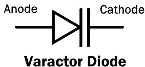
Figure1. 39Varactor Diode
