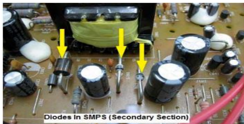
Figure2.74. Secondary Output Diode
