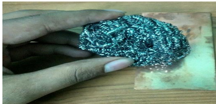
Figure 2.44 Scrub the copper
