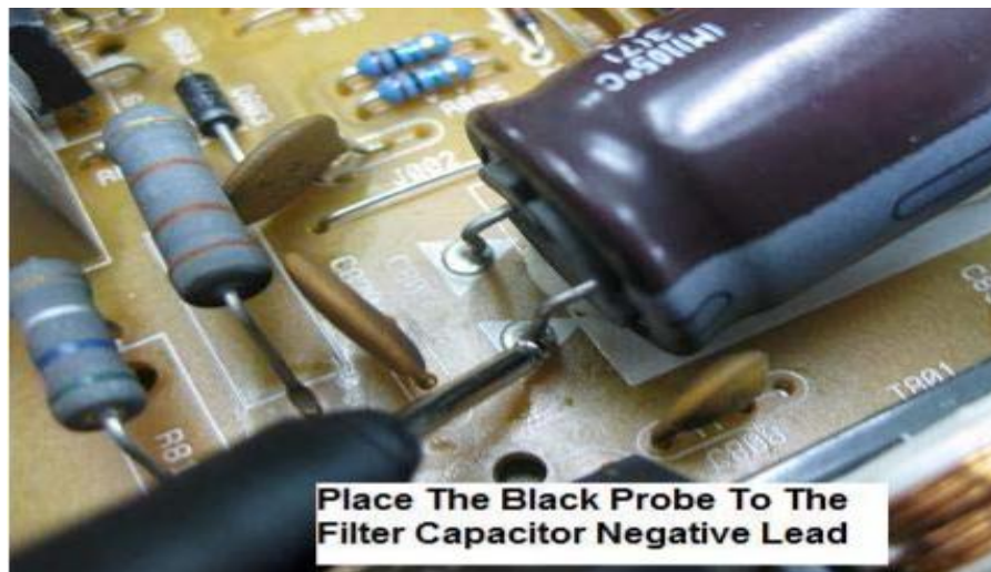
Figure2.100 Placing the BLACK test probe to the negative pin of the Filter Capacitor.
