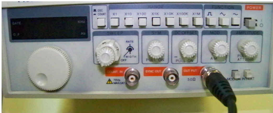
Figure1. 55Signal Generator
