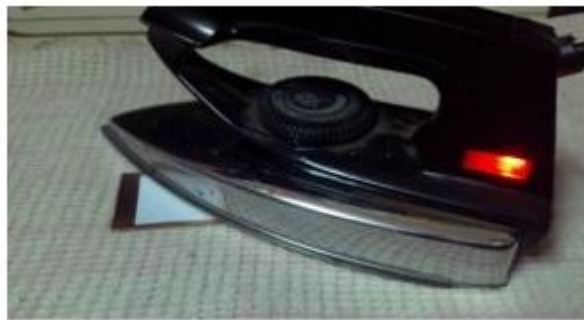
Iron the paper onto the plate
