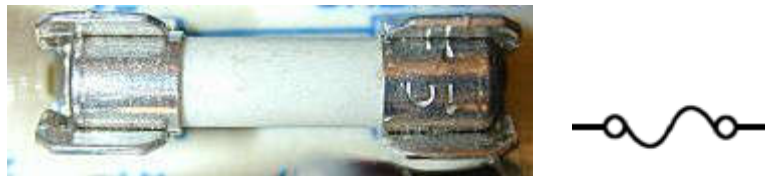
A fuse, sitting in its fuse holder, from the interior of a PC power supply.
