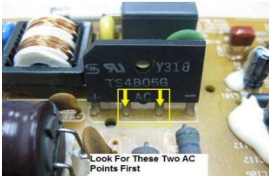
Figure2.96. Two AC Pins of a Bridge Rectifier on a Single Package.
