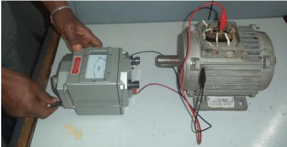
Figure 3.12 insulation resistance testing
