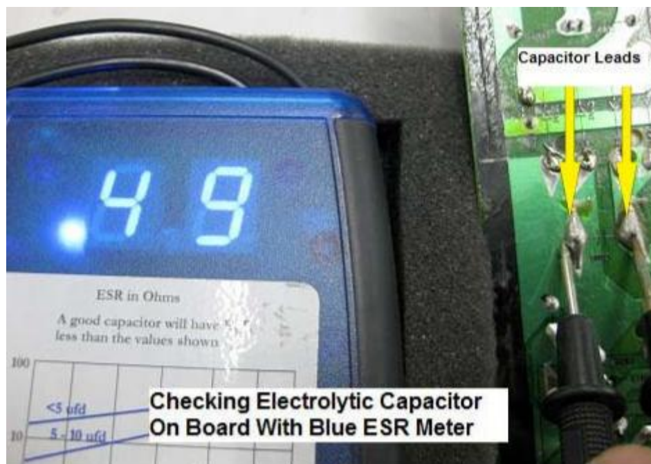
Figure3.14. Checking the electrolytic capacitor using Blue ESR meter
