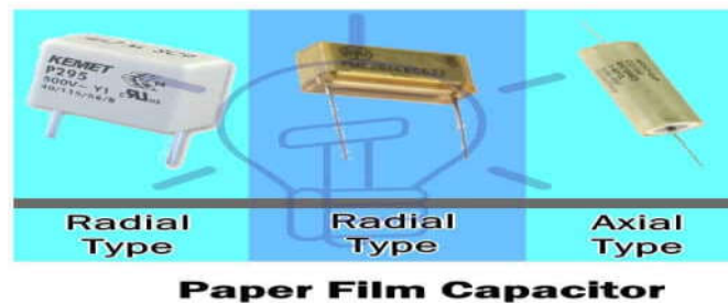
Figure1. 29 Paper Capacitors
