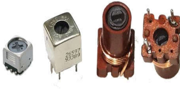
Figure1. 14Variable Inductors
