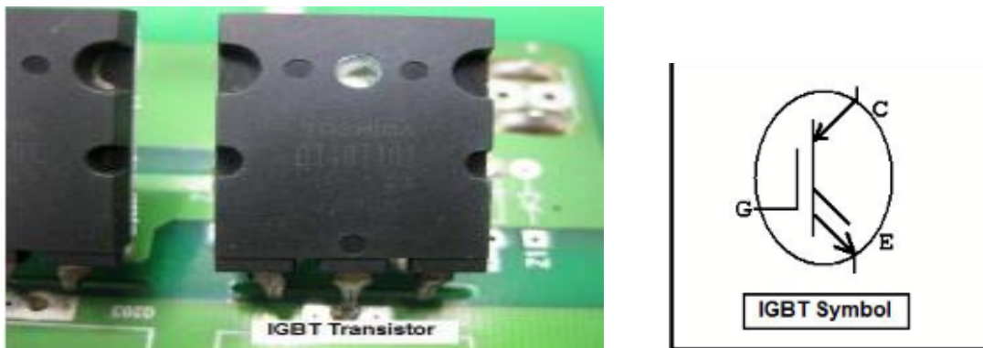
Figure2.69. IGBT Transistor and Symbol
