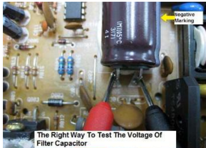
Figure2.98 Testing voltage at the filter capacitor
