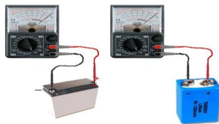
Figure2.7. Caution in measuring resistance
