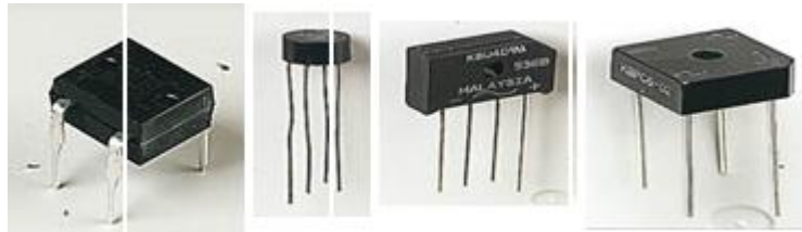
Figure 2.23 various types of Bridge Rectifiers
