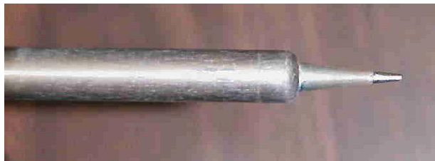
Figure 2.53.A properly cleaned and “wetted” soldering iron tip.
