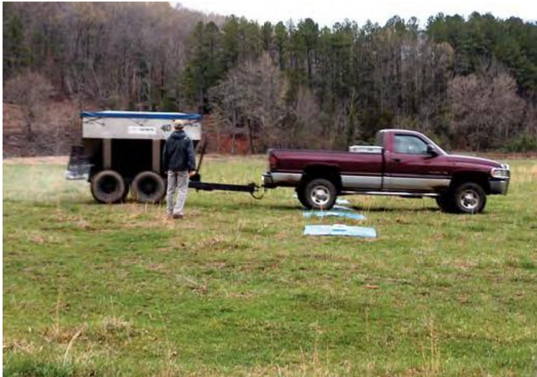
Figure 4. A farmer calibrates a fertilizer spreader before fertilizing to ensure delivery of the intended fertilizer rate to the pasture
