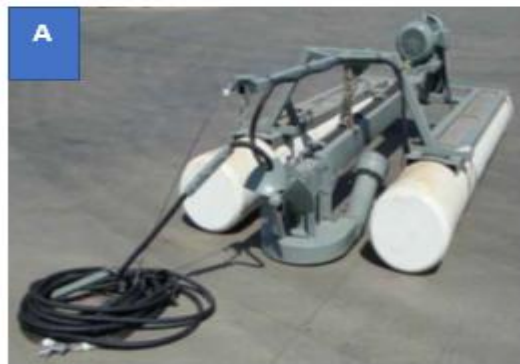
Figure 31-A: Float-mounted agitator pump and Figure 31-B: Open-impeller agitator
