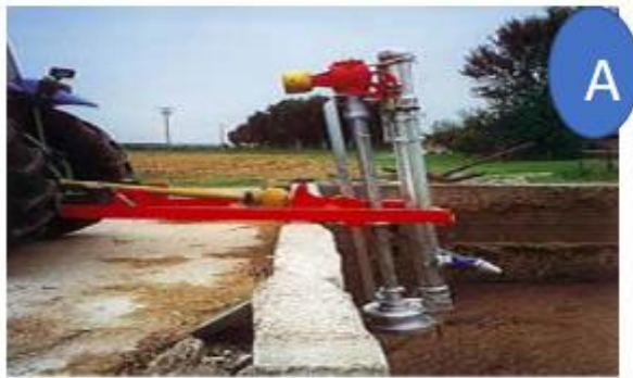
Figure 30-A: Vertical shaft PTO-powered chopper-agitator Pump and Figure 30 -B: Vertical shaft chopper-agitator pump with
