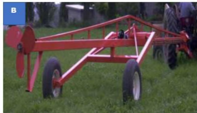
Figure 31-A: Float-mounted agitator pump and Figure 31-B: Open-impeller agitator
