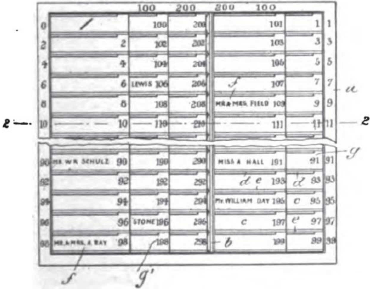
Figure no 5.5 room rack frame with flexible card holders mounted on pivots
