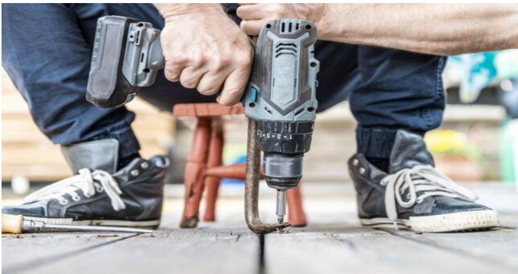
Figure 1. 88 Try a left-handed drill bit
