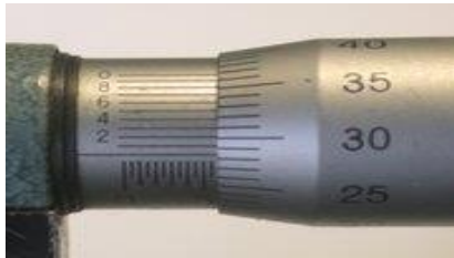
Figure 1. 33 E Vernier Micrometer
