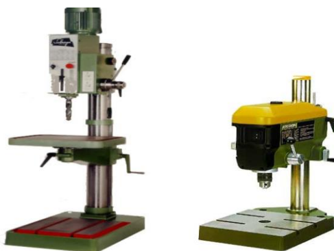
Figure. 1.10 Press drill Machine
