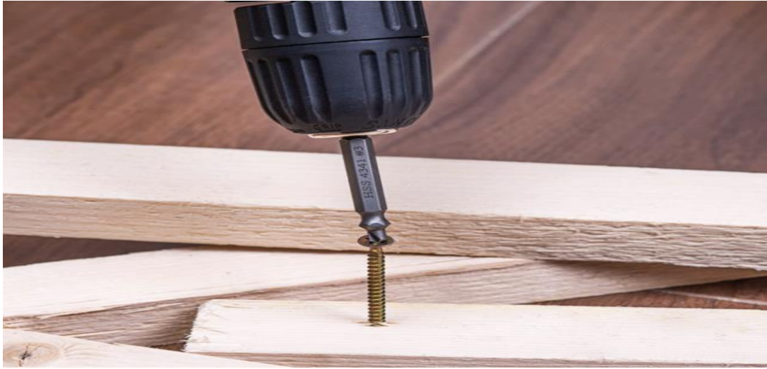
Figure 1. 87 Use a stripped screw extractor
