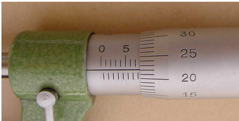
Figure 1. 30 B The reading is 7.72 mm.
