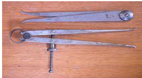
Figure 1. 15 Inside calipers
