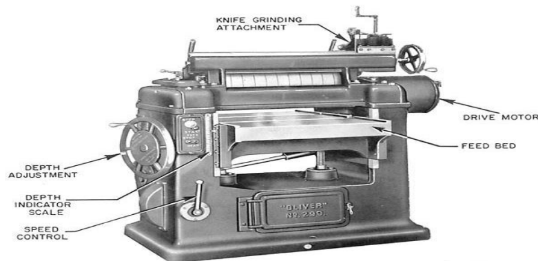
Figure 15 how a planner works
