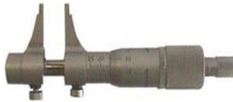
Figure 1. 31 C inside Micrometer
