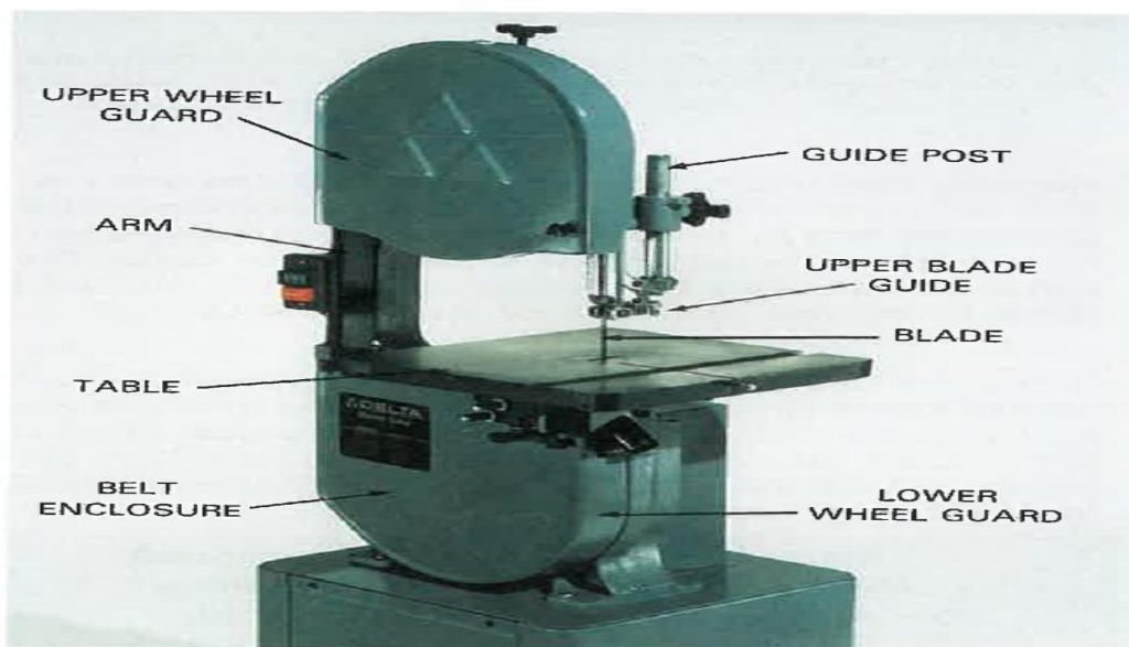
Fig. 15-1. Parts of a standard band saw. (Delta International Machinery Corp.)
