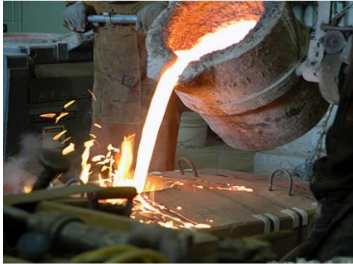
Figure 1.7 Atypical gravity casting pouring process
