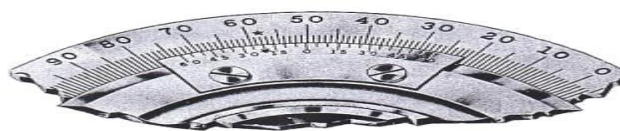
Fig. 6.1.9 Reading the size of an angle of vernier bevel protractor
