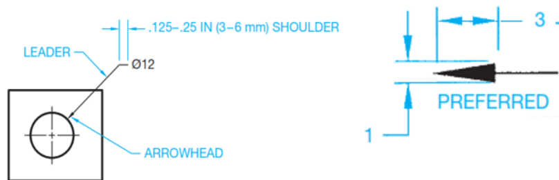
Figure 2.7 Leader line with its arrow head
