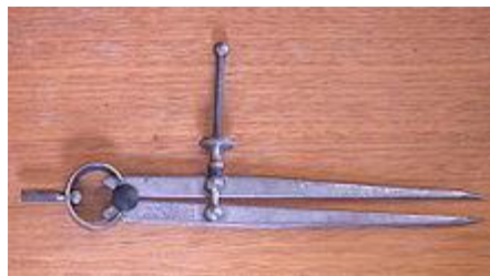
Figure 1. 17 divider calipers
