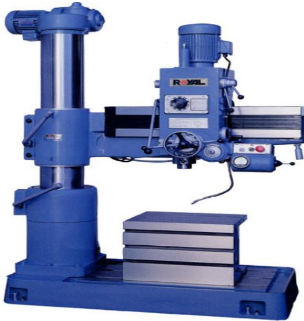
Figure. 1.11 Radial drill Machine
