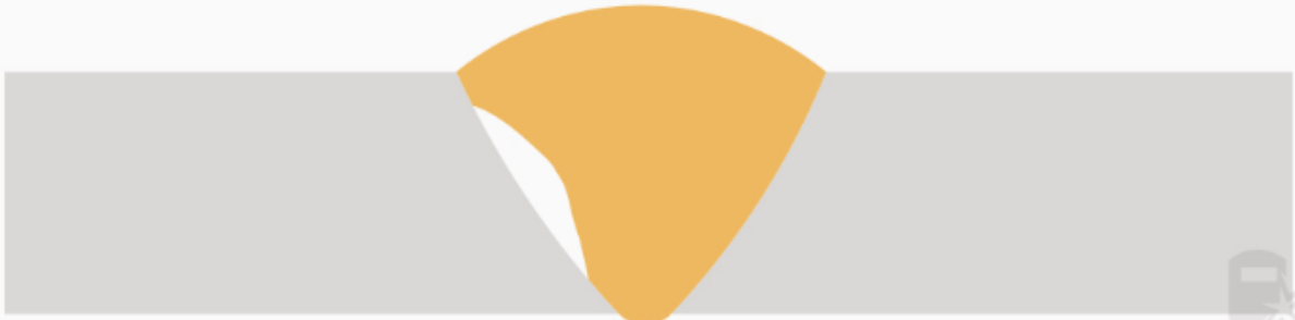
Figure 5.2 Figure 38 Lack of Fusion
