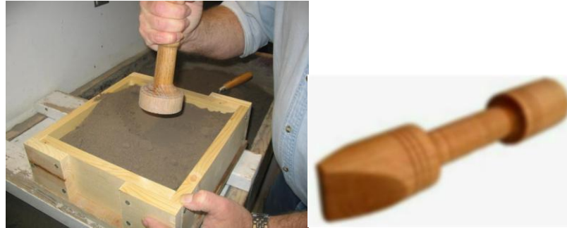
Figure 3. 11 Ramming the Sand
