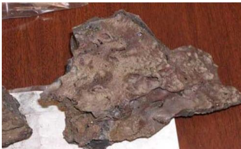
Figure 3.19 A typical slag sample from a coal-fired steam generator.
