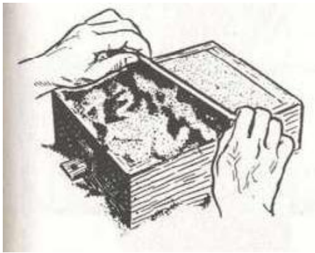
Figure 3.7 Venting with pointed wire
