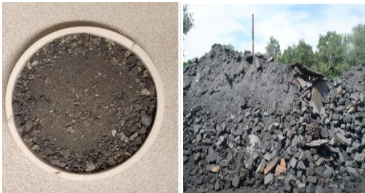
Figure 2.3 Disposing of damaged refractory materials
