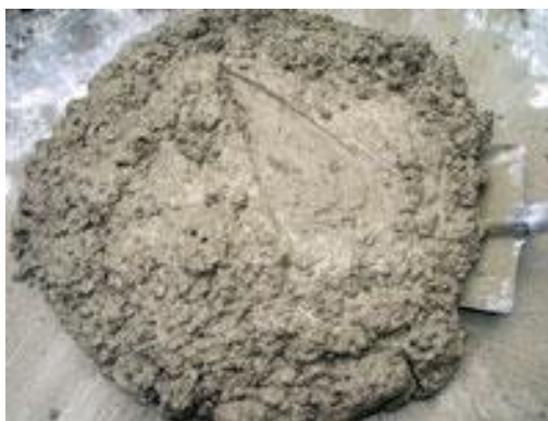
Figure 3.18 Refractory concrete of good consistency
