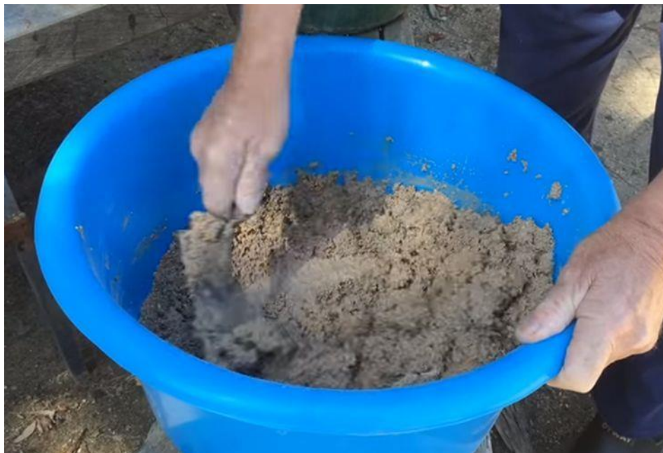
Figure 3.12 hand mix of Heat resistant refractory concrete
