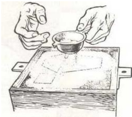
Figure 3.9. Dusting with parting powder
