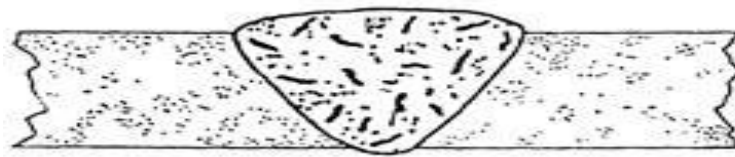
Figure 5.4 Slag Inclusion
