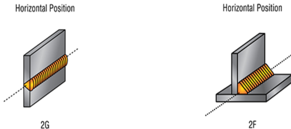
Figure 4.3 Scheme of placement of components to be welded for horizontal welding
