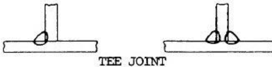
Figure 1.15 Tee Joint
