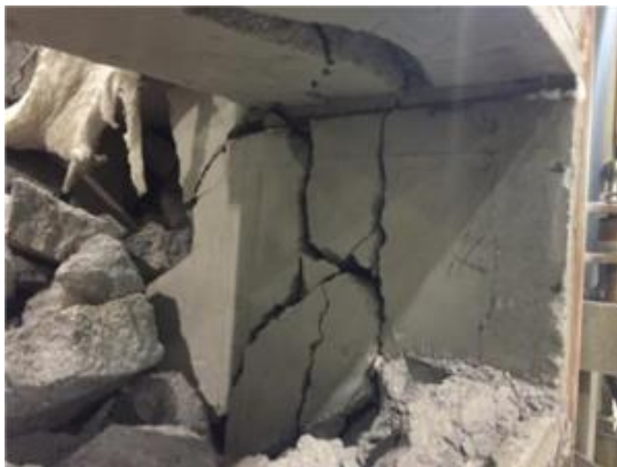
Figure 4.1 Failure to properly mix, place, and cure refractory materials along with using improper dry out schedules or practices can result in severe spalling
