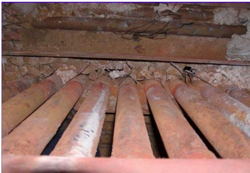
Figure 3.21 The refractory seals inside this furnace failed and must be replaced.
