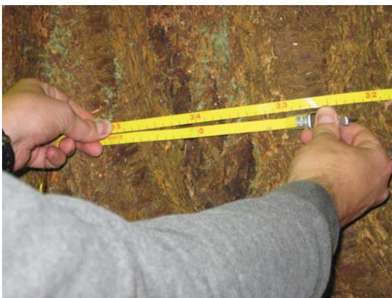
Figure 24: A diameter tape is graduated so that diameter can be read from measuring the tree's circumference.
