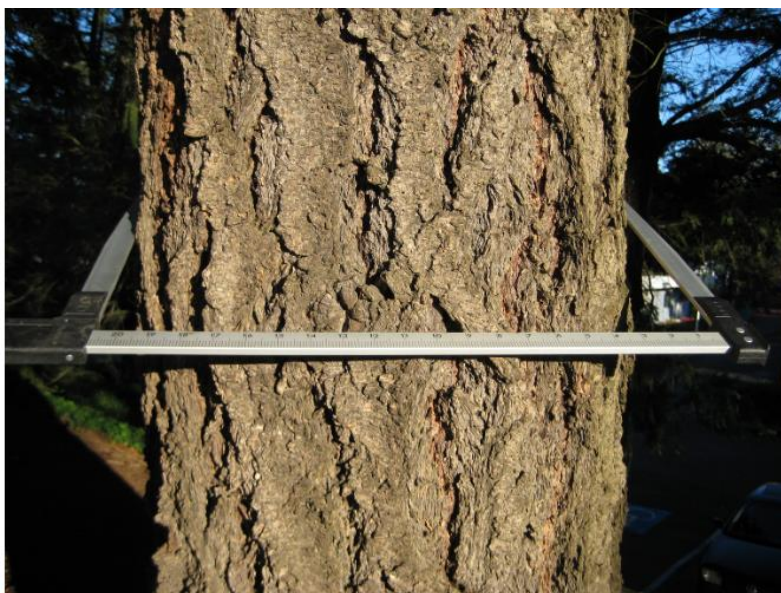
Figure 23: A tree caliper is held at right angles to the tree trunk.
