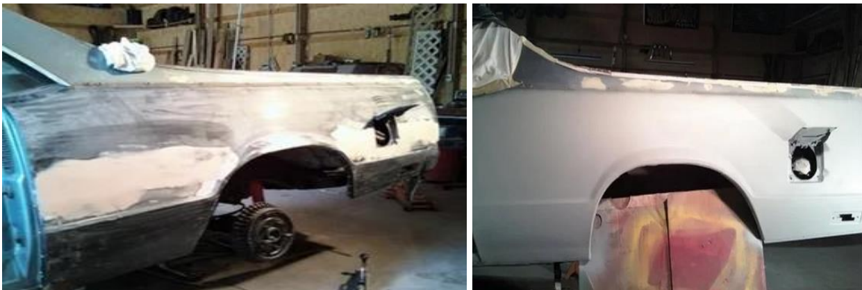
Figure 5: Sanding the Panel after applying putty
