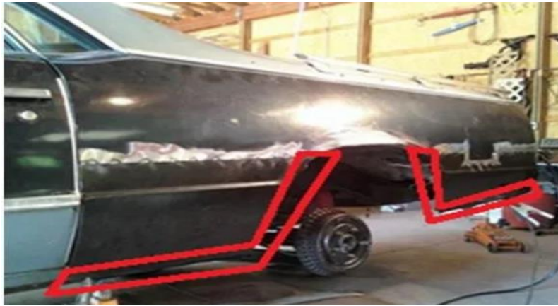
Figure 3: Attaching the Panel bottom part.
