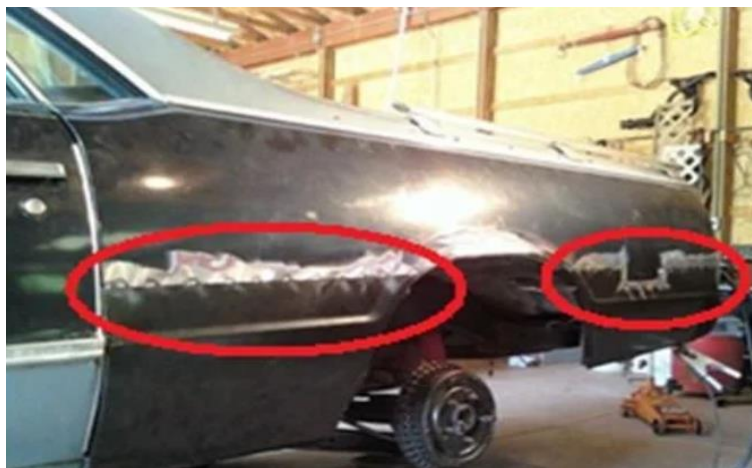
Figure 2: Welding prepared panel with vehicle body
