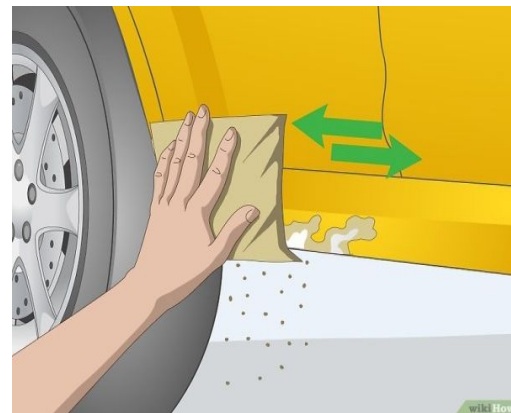
Fig:4. Sand the area to prep the surface
