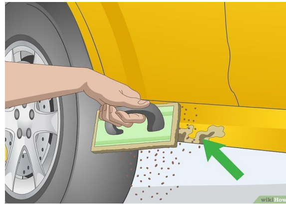
Fig: 2. Check for rust and remove
