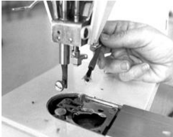
Figure 1.5: Cleaning bobbin area
