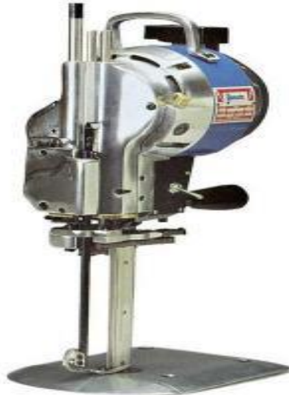
Figure 3.17: Straight knife cutting machine
