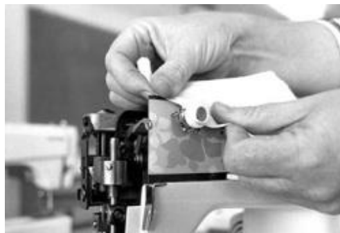
Figure 1.4: upper thread tension
