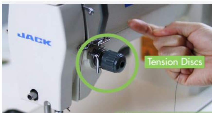
Figure1.9: tension disc
