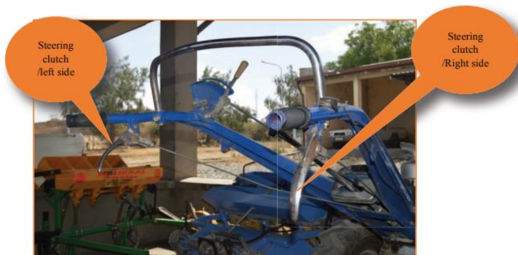
Figure 3:1 walking tractor steering clutch (left & right sides).
