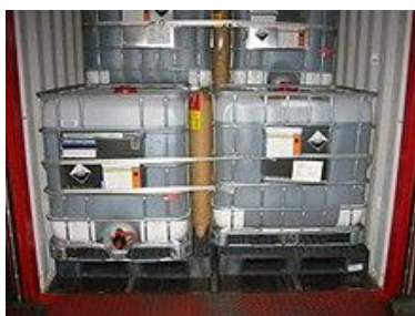
Figure 6.5. Polyester strapping and dunnage bag application
