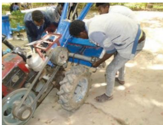
Figure 4:7. Mounting the seeder to the drawbar pull/gearbox of the walking tractor
