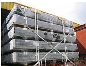
Figure 6.6. Polyester Lashing application
