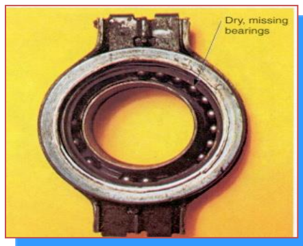
Figure 2.3(f): Dry Release Bearing
