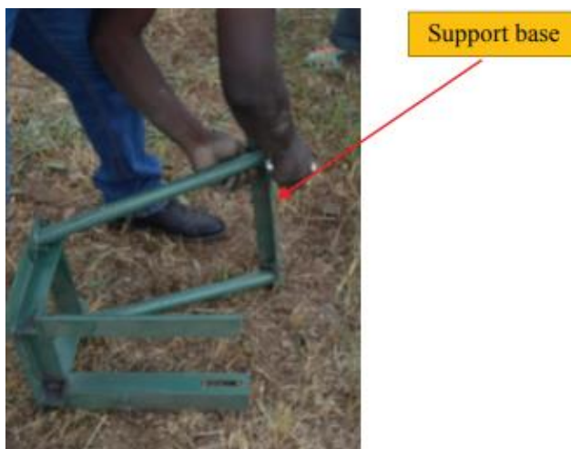
Removal of the securing bolts
