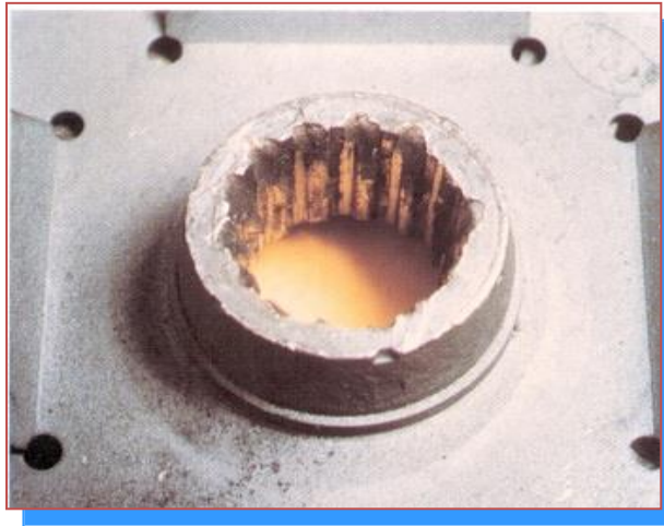
Figure 2.3(e): Damaged Hub Spines
