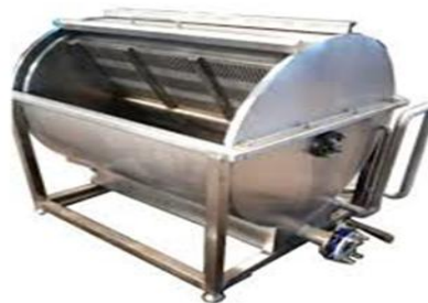
Figure 2.5: Rotary poultry scalding machine for poultry abattoir
