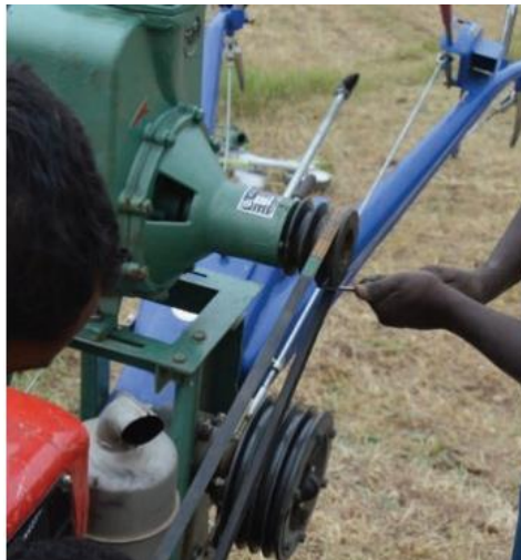
Inserting a v-belt from the engine pulley side and then from the clutch pulley
