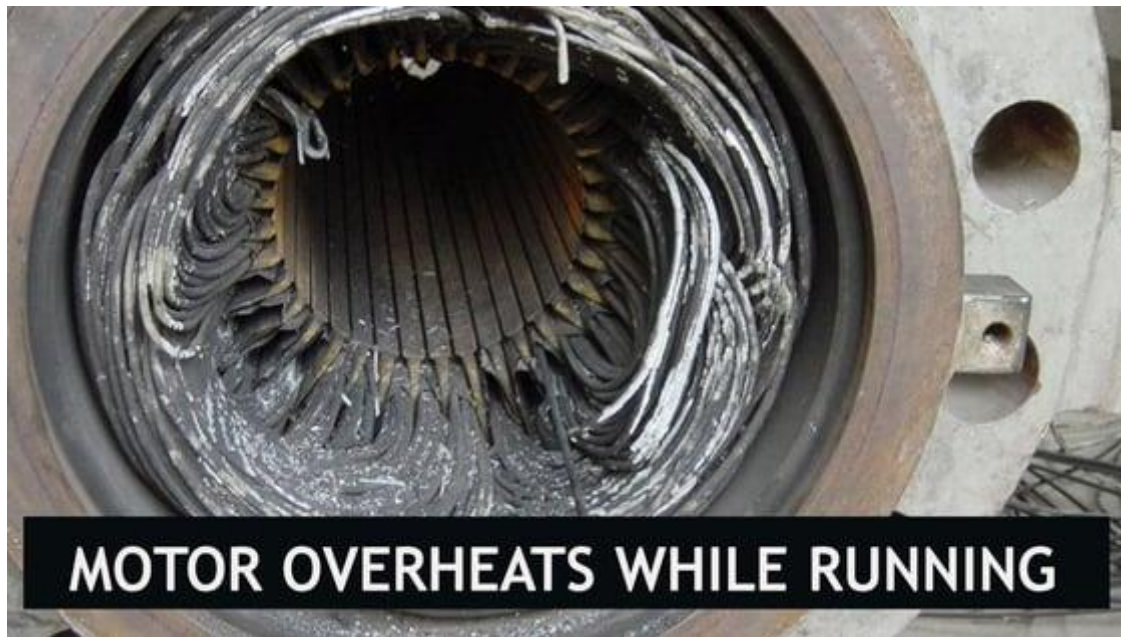
Figure 2.25 electric motor stator that has experienced extreme heat damage
