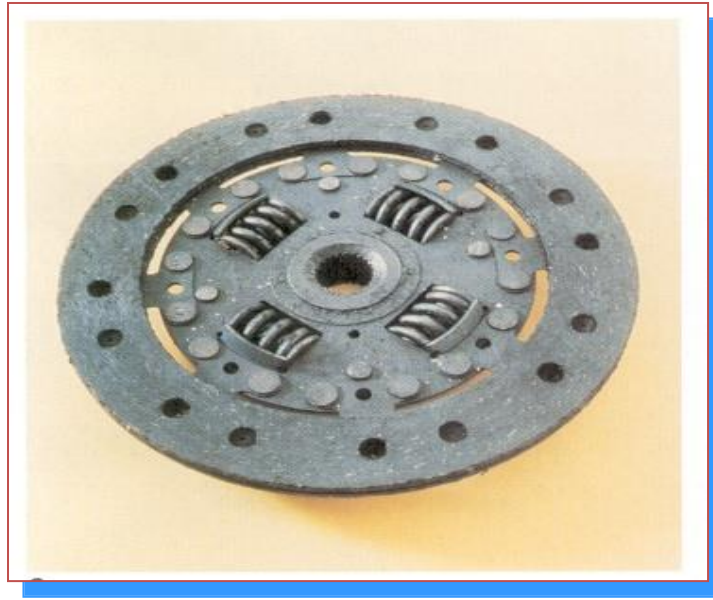
Figure 2.3(c): Burned Clutch Disc
