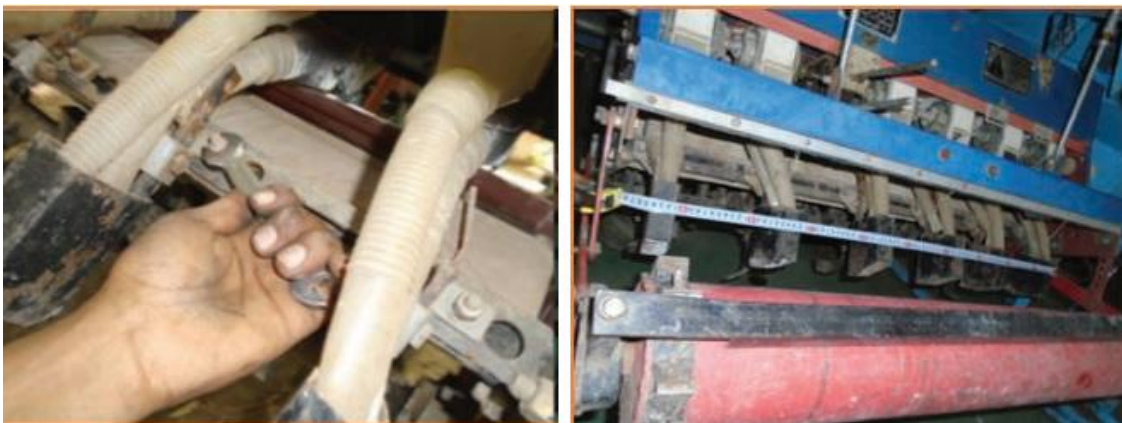
Figure 4:26 adjusting furrow opener spacing
