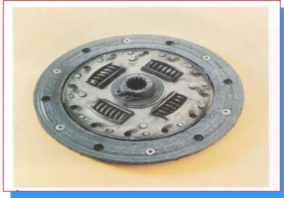
Figure 2.3(a): Worn Clutch Disc
