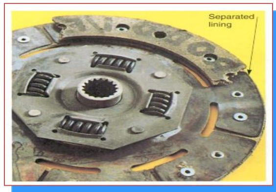
Figure 2.3(b): Separated Lining
