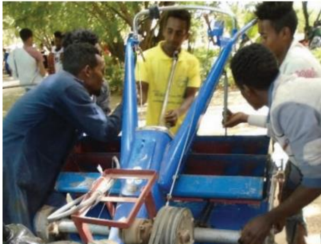
Figure 4:8. Mounting levers to attach the planter to walking steering column
