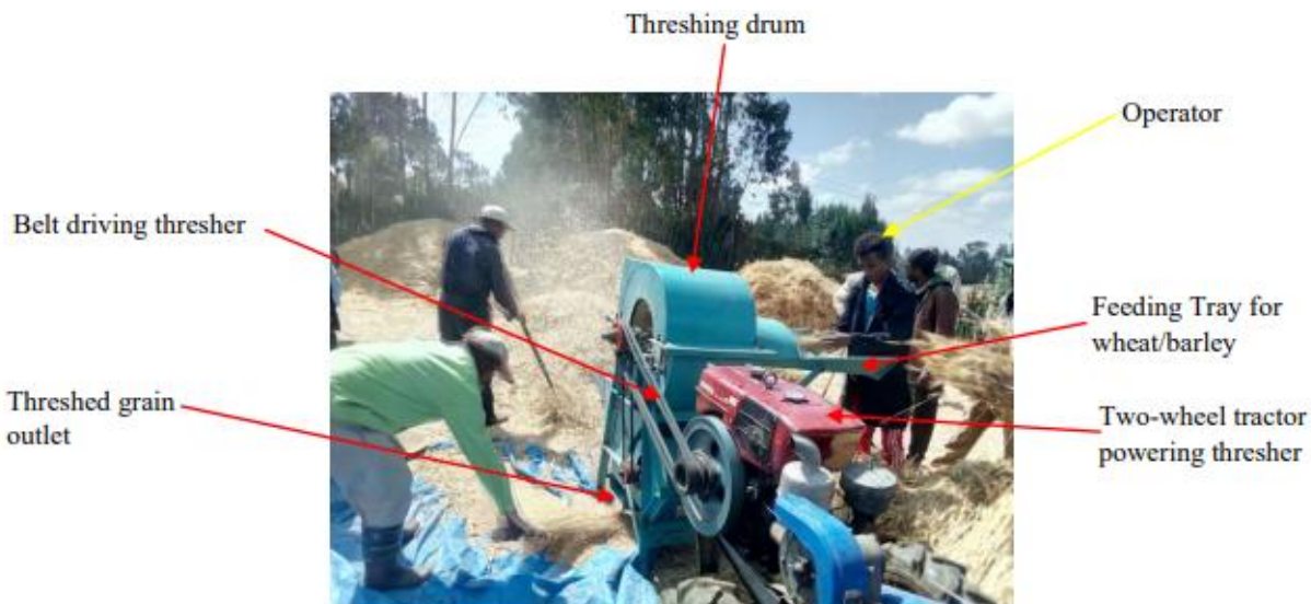
Figure 5:9 Thresher/Sheller parts and Operation system
