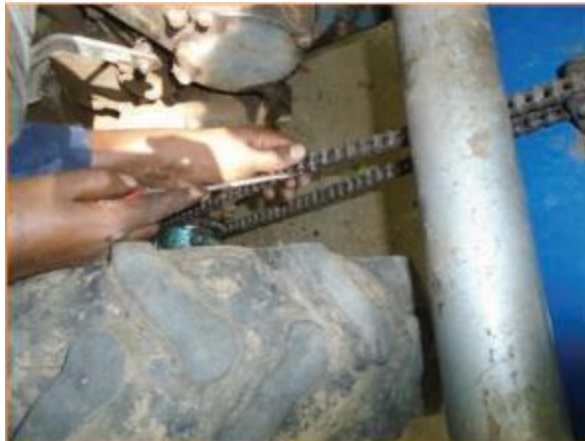
Figure 4:9. Alignment of sprockets and chain
