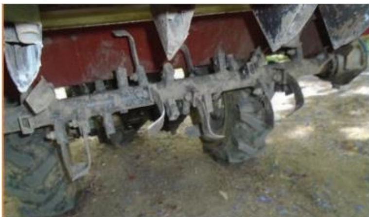
Figure 4:4. Installed blades on the rotavator's shaft
