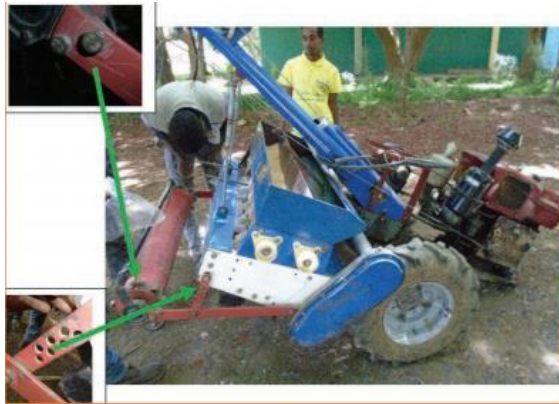
Figure 4:5. Assembling press wheel/roller
