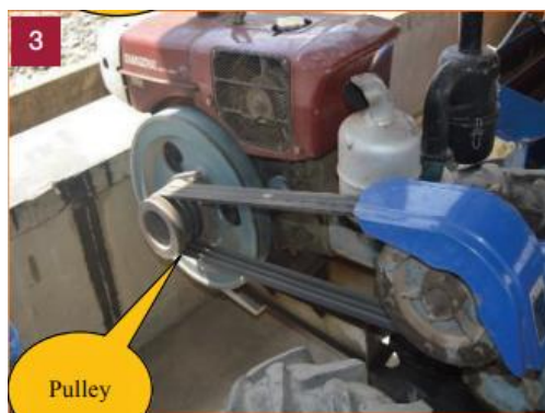
Figure 4:1. Method of fitting attachment to walking tractor
