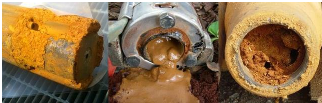
Figure 2.23 Fouled pumps and irrigation lines.
