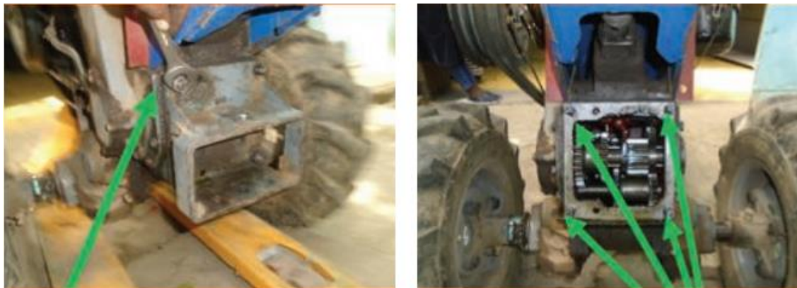
Figure 4:6. Removing drawbar pull cover
