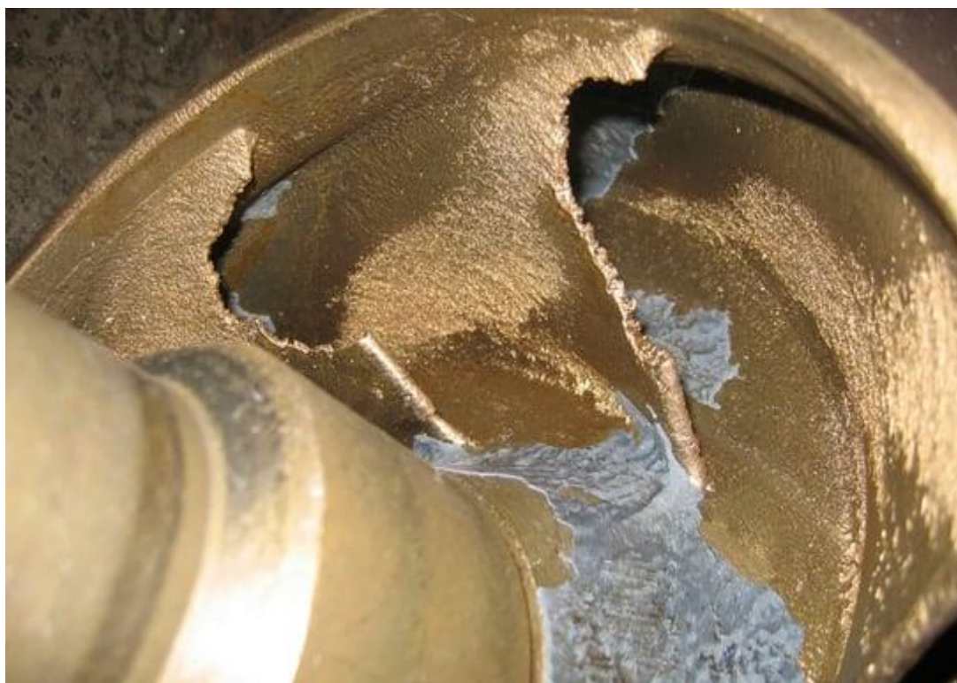
Figure 2.22 Impeller damage from cavitations
