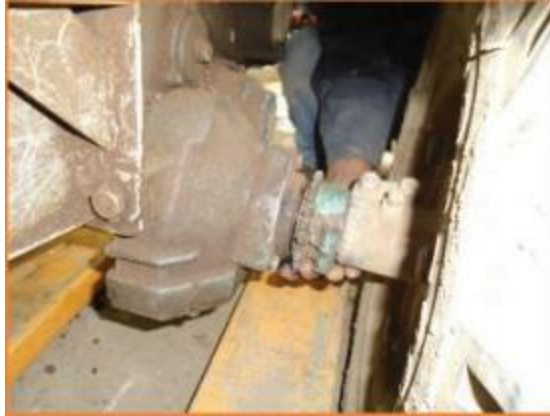
Figure 4:2. Inserting the drive sprocket to the drive axle
