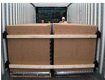
Figure 6.4. Blocking and bracing with timber
