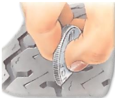
Figure 7.1. Checking tractor tread
