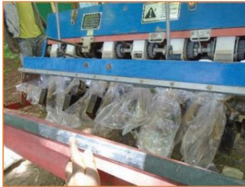
Figure 4:27 attaching transparent polythene bags to each of the six seed delivery tubes.
