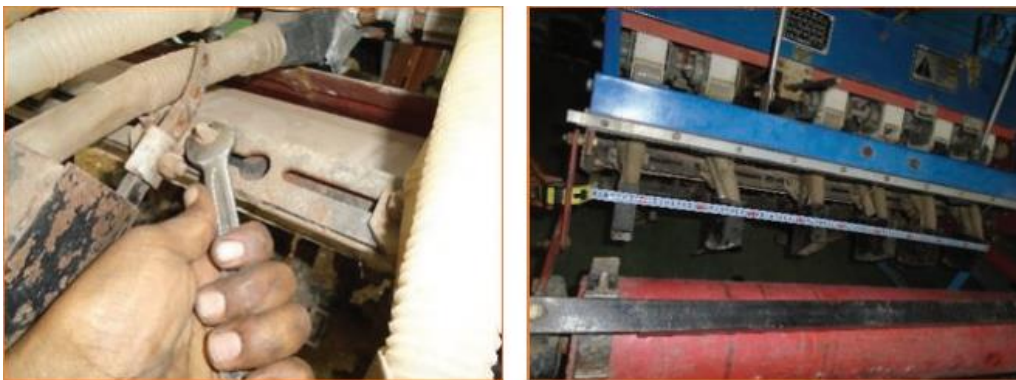
Figure 4:3. Assembling of furrow openers
