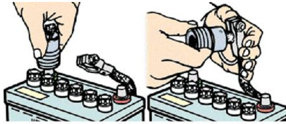
Figure 2.7: battery terminal cleaning
