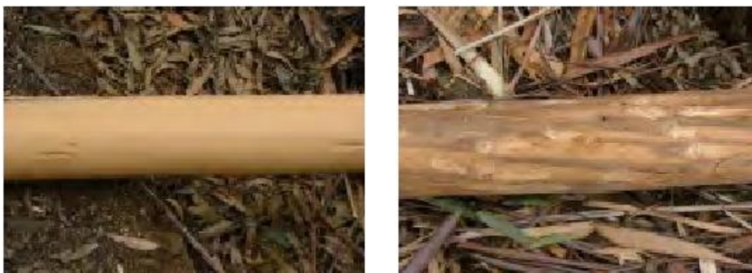
Figure 24left: Cleanly stripped log, right: Chiseled log.
