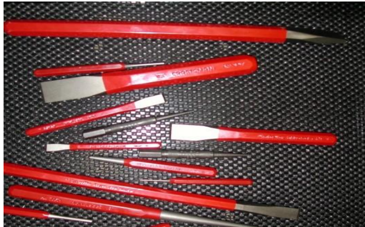
Figure 1.1 Chisels
