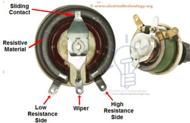
Wire wound Rheostat Construction
