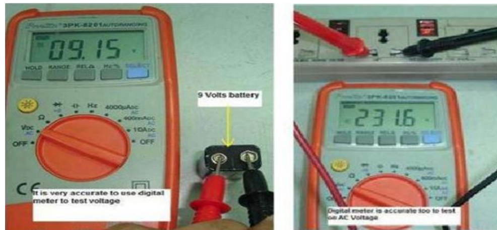
Figure 6.5 Measuring the voltage using digital meter.
