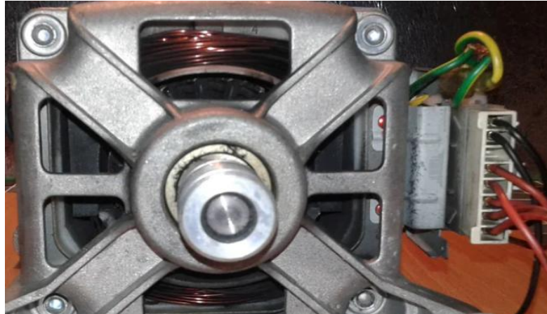
Figure 2.16 universal motor
