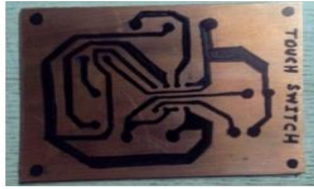
Using the permanent marker for sketching the PCB
