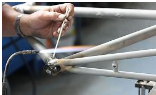
Figure 3.9 Hard Soldering
