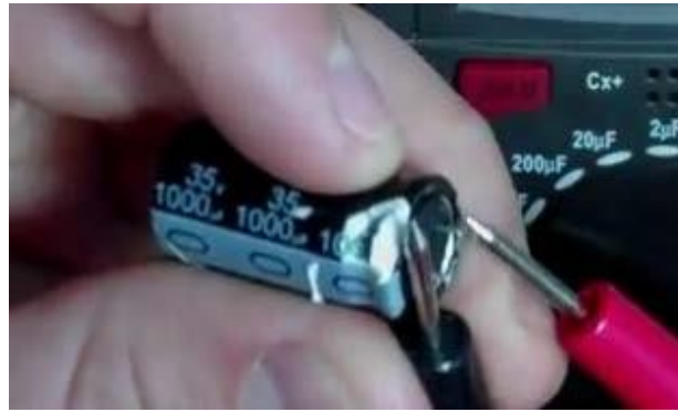
Figure 2.7 connections of capacitor and meter
