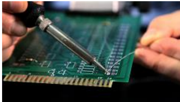
Figure 3.8 Soft Soldering
