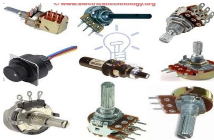
Figure 1.43 Different Types of Potentiometers
