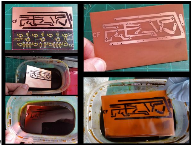
Fig.2.3. PCB etching process
