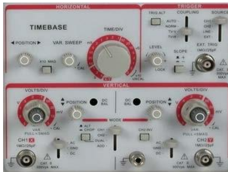
Figure 1.13 Controls of Analog Oscilloscope
