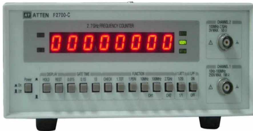
Figure 1.27 Frequency counter
