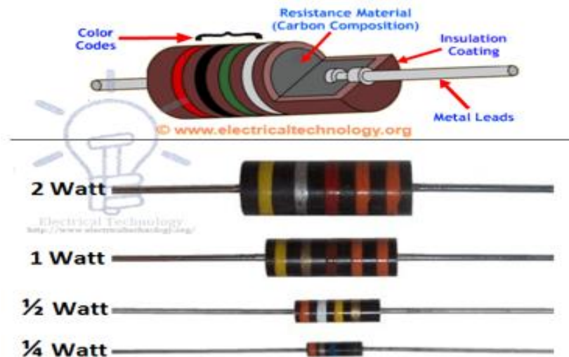
Figure 1.37 Constructions and Wattage Rating of Carbon Composition Resistors.
