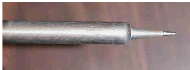
FIG 3.5.1. A properly cleaned and “wetted” soldering iron tip.
