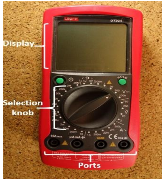
Figure 2.4 Parts of a Digital Multimeter
