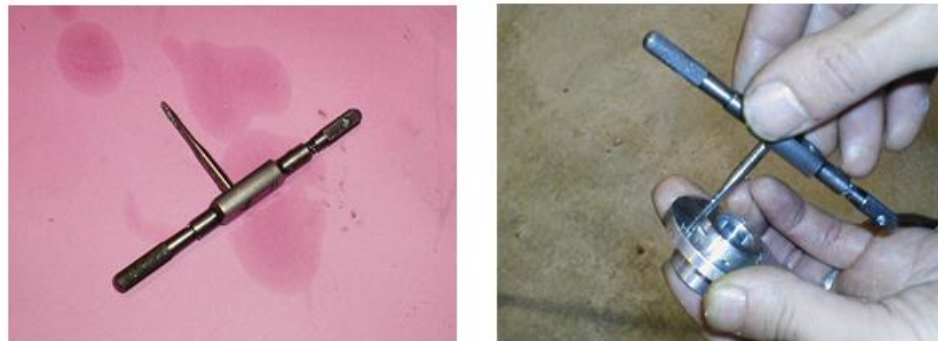
Figure 76: A Tap with a Tap handle and Thread Cutting using a Tap
