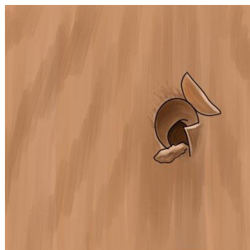
Figure 93: burrs on wood
