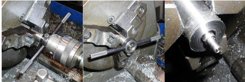
Figure 81: Thread making using die
