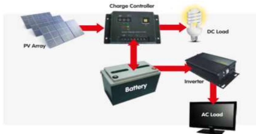
Figure 4: schematic of stand-alone PV system with battery storage powering DC and AC loads
