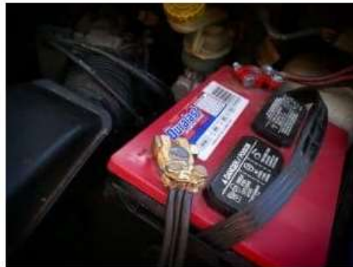
Fig corroded battery terminals
