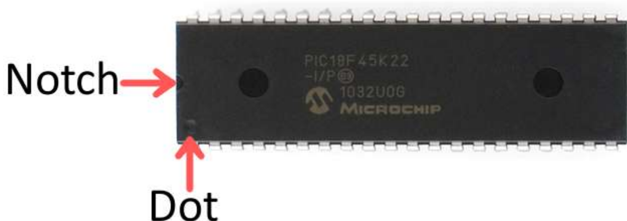
Fig 3.8. Polarity and pin numbering of ICs
