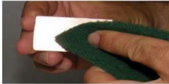
Rubbing away the top oxide layer
