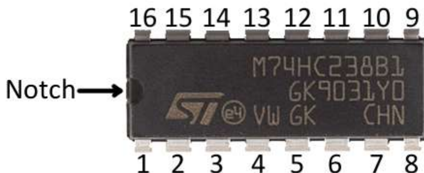
Fig 3.9. Polarity and pin numbering of ICs
