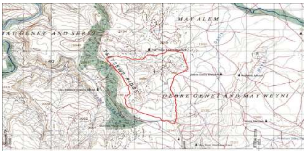
Fig: conventional method of delineation of area to be assessed & measured using a topographic map.
