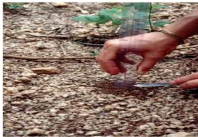
PHOTO 25 Removal of a portion of an armour layer. (Stocking and Murnaghan, 2001)
