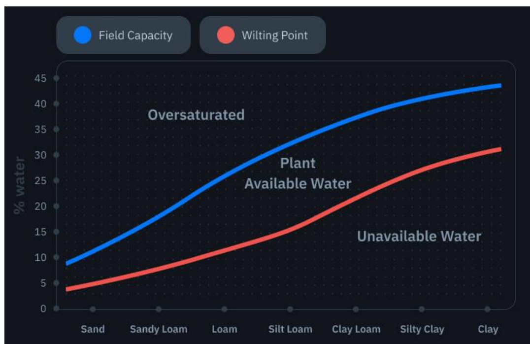
Figure 2.2. Optimum moisture content of soil
