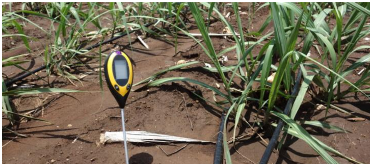
Figure 2.3. Measuring soil moisture using digital soil moisture meter
