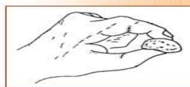
Plastic Limit (PL) determination of fine soil
