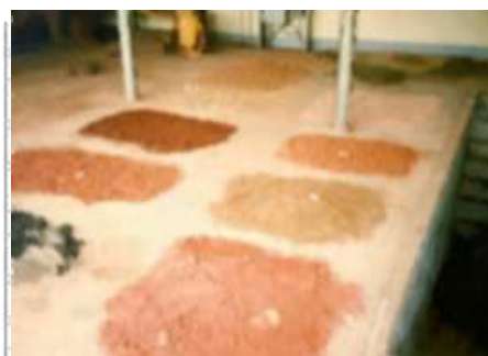
Samples drying under cover prior to testing
