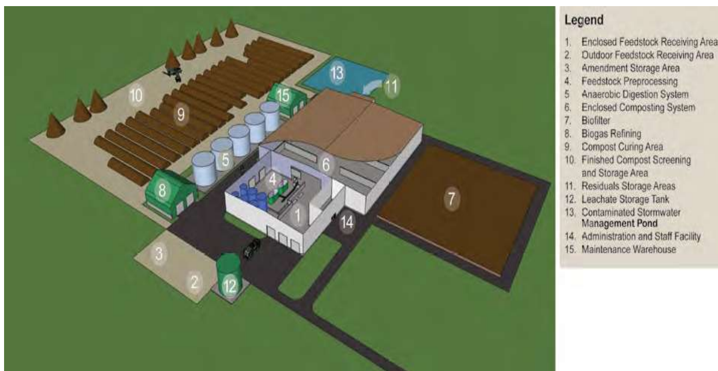
Figure 5.1. Operating areas in typical solid waste organics processing facility
