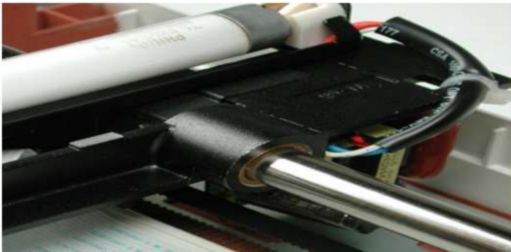
Fig 1.25 The stabilizer bar is very durable and tightly secured to the body of the scanner.
