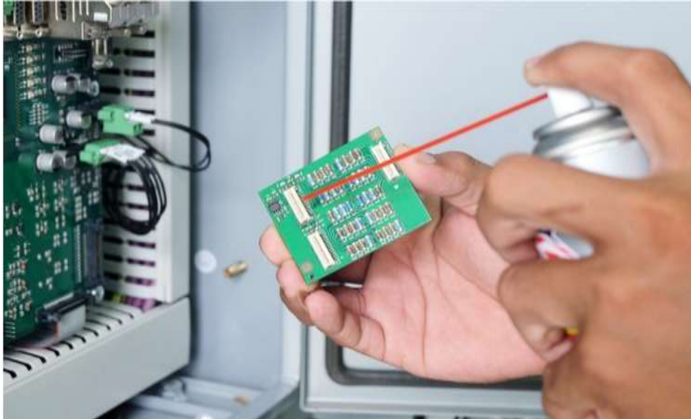
Fig 6.2 cleaning a circuit board
