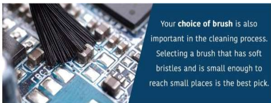
Fig 6.3 using brush to clean PCB
