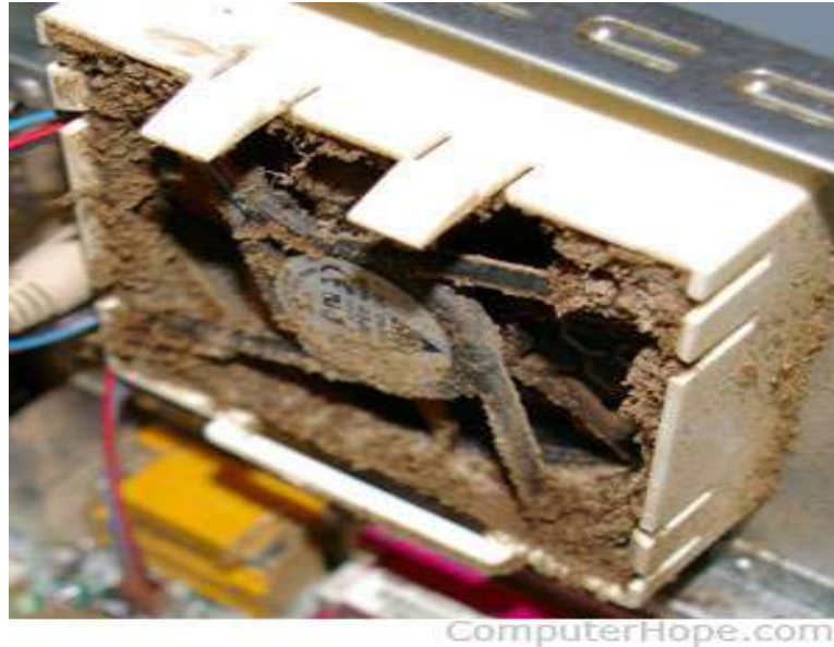
Fig 3.1 dust inside computer
