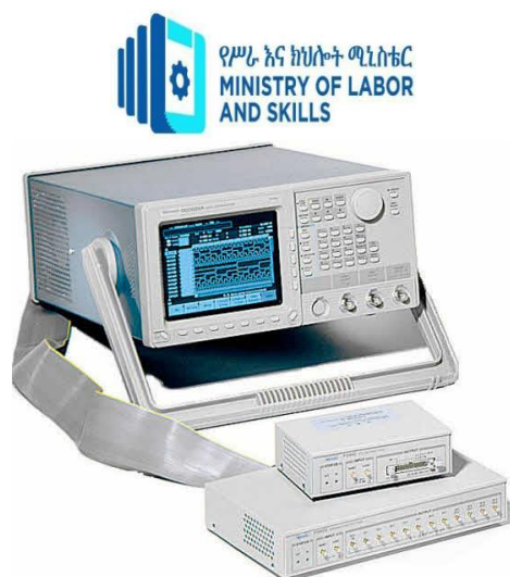
Figure 1.6 Digital Pattern Generator
