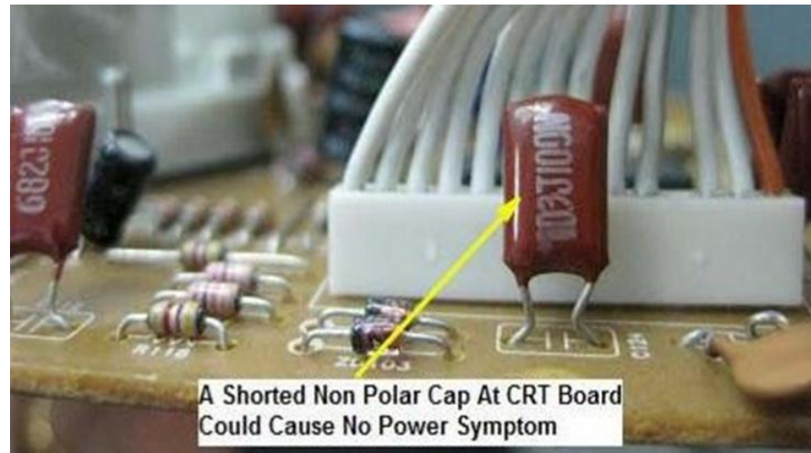
Figure 3.11: Shorted Non Polar Capacitor at CRT Board
