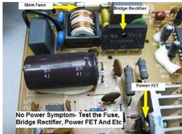
Figure 3.1: Basic Way of fault finding for no power
