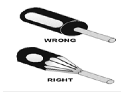
Figure 1.17: Knife Stripping
