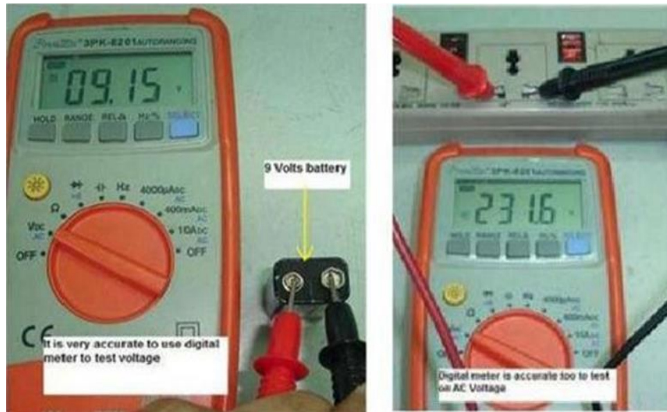
Figure 2.4: Measuring the voltage using digital meter.
