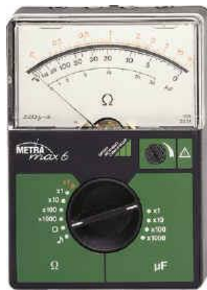
Figure 1.2 ohmmeter
