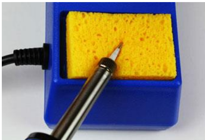
Figure: Tinning the Tip
