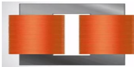
Figure: Core type transformer
