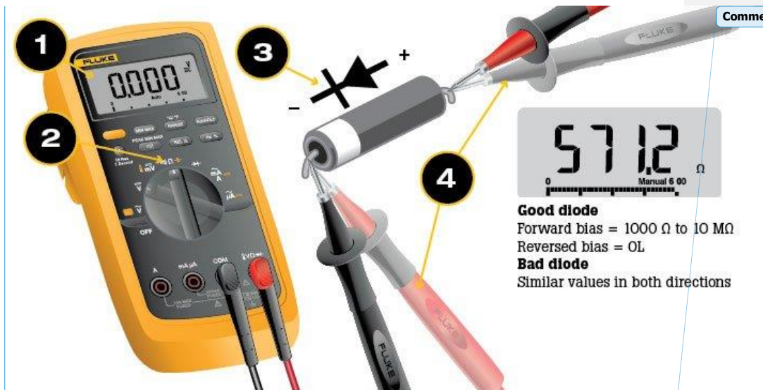
Figure 3.2: Resistance mode diode testing
