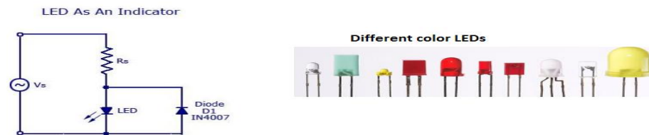
Figure: LED Circuit
