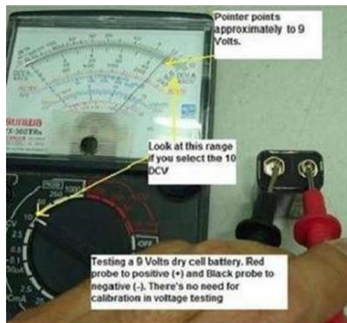
Figure2: measuring the voltage using analogue meter
