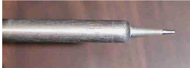
Figure 2.4: A properly cleaned and “wetted” soldering iron tip.
