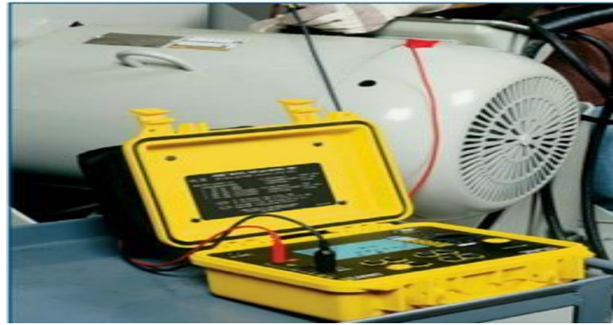
Figure 59: Measuring insulation resistance
