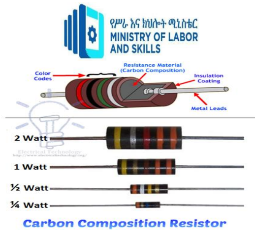
Figure:carbon composition resistor
