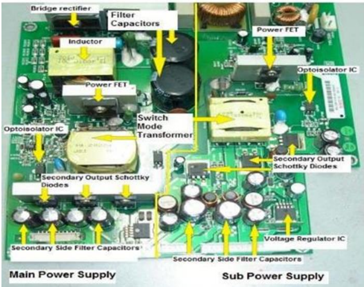
Figure 1.40: typical LCD Monitor SMPS
