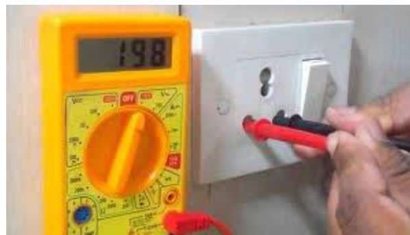
Figure 2.6: Measuring Voltage from single-phase power outlet
