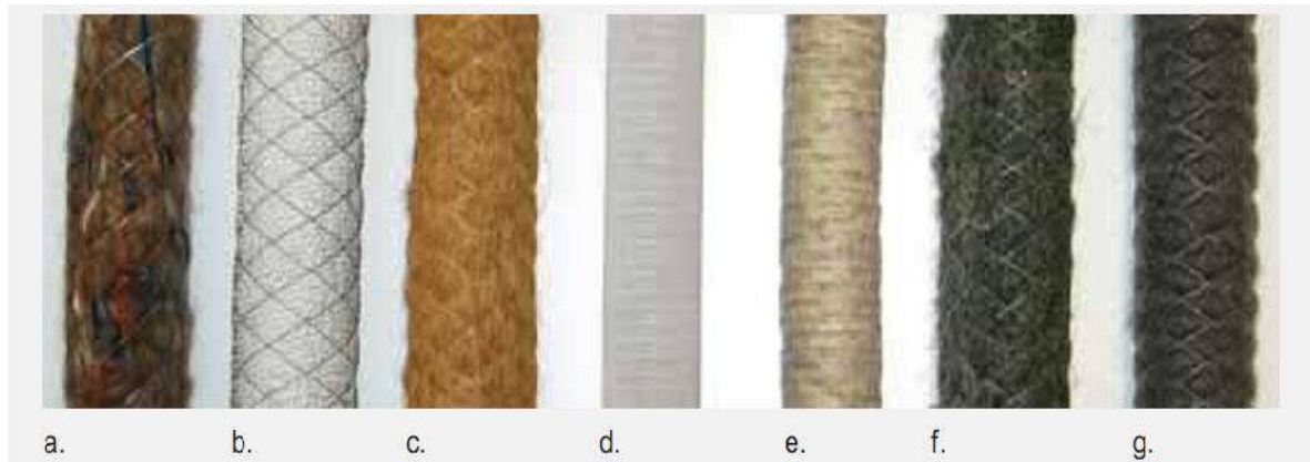
Figure_7: Envelopes can be made of wrapped polypropylene fibers (a, f & g), polystyrene granules (b) and coconut fibers (c), non-woven nylon (d) and woven type (e)
