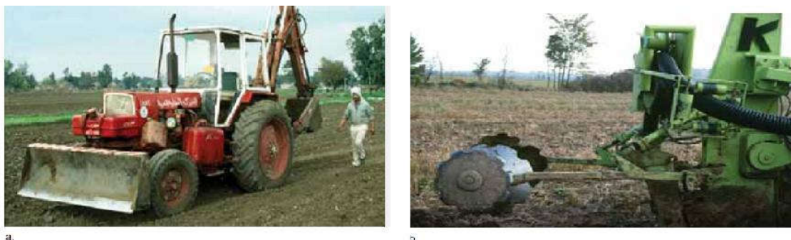
Figure_10: Backfill equipment: tractor with dozer blade (a) and V-shaped disc-blade mounted at the rear end of a subsoil type trenchless drainage machine (b)
