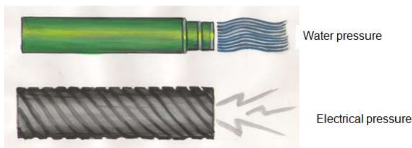
Figure 2: Similarity of water pressure and Voltage
