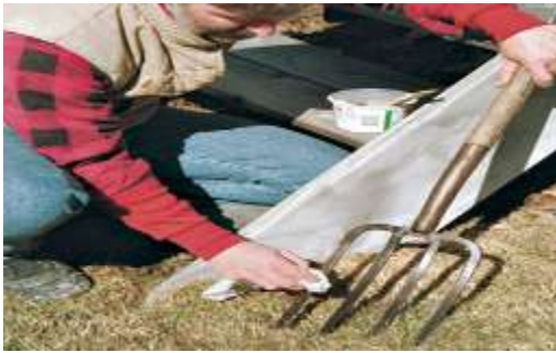
Fig.2 Oil steel tool heads to prevent them from oxidizing. The oil creates a barrier between the air and the steel.
