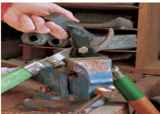
Fig.7 Sharpen pruning blades and knives by sliding an oiled honing stone in one direction across the tool's beveled edge.
