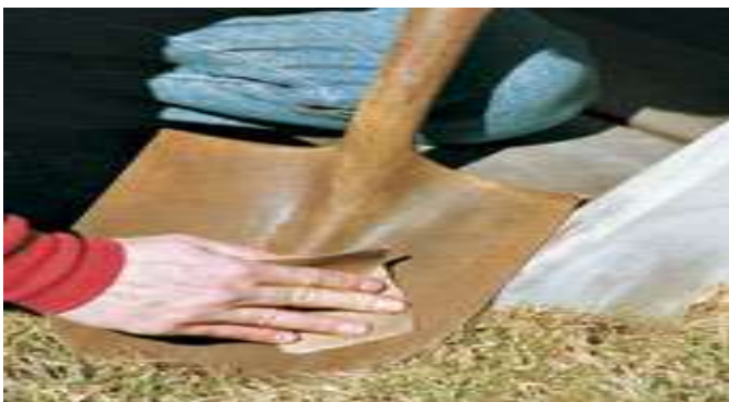
Fig.3 Sand away a light coating of rust. 80-grit sandpaper should be coarse enough to get the job done.
