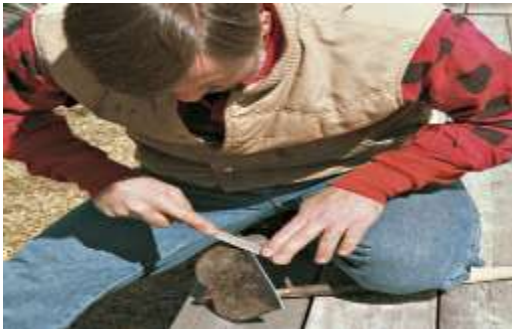
Fig.6 Use a hand-held mill file to sharpen hoes and shovels. The key to successful sharpening is keeping the tool steady and the file at the proper angle.
