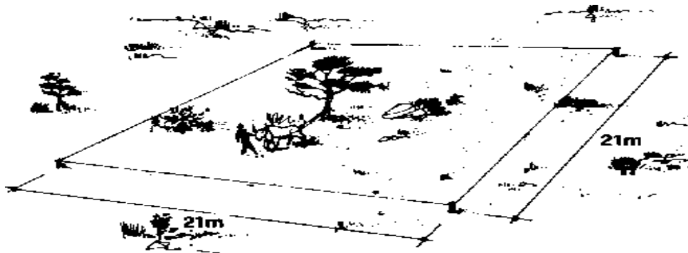
Figure 2.8. Measuring and marking the selected site for construction
