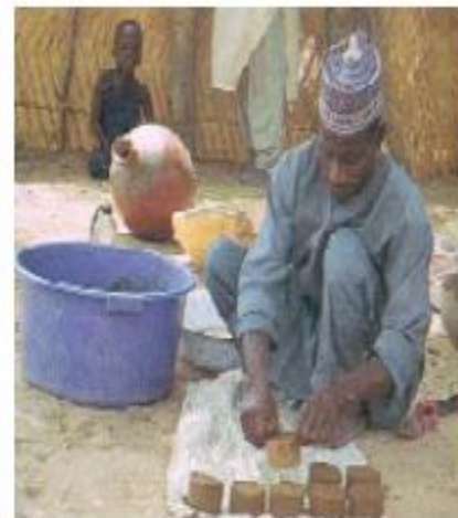
Removing molded blocks for drying
