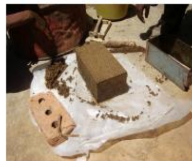
Step 5. UMB ready for drying
