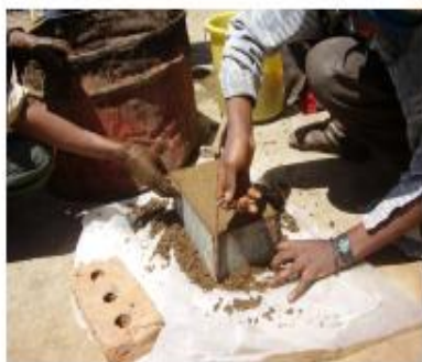
Step 3. Opening the mold
