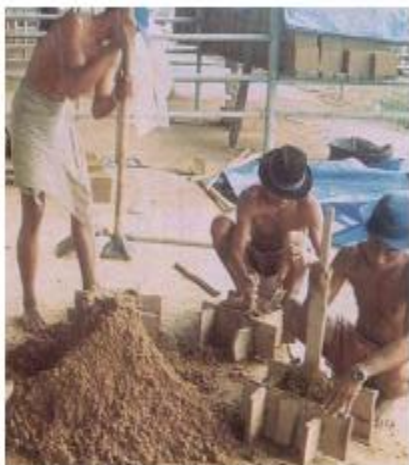
Molding using wooden bars
