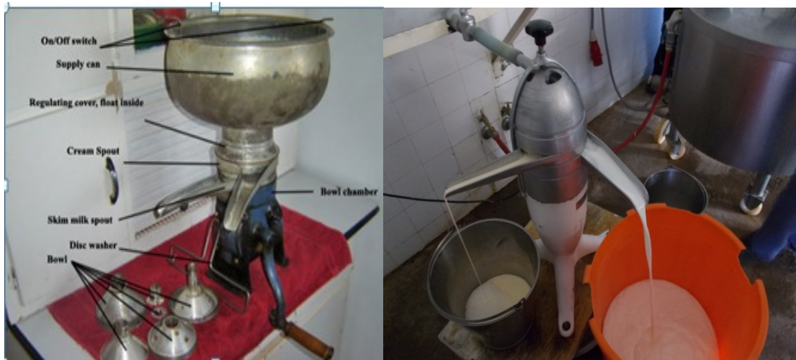
Figure 2.7: Centrifugal cream separator
