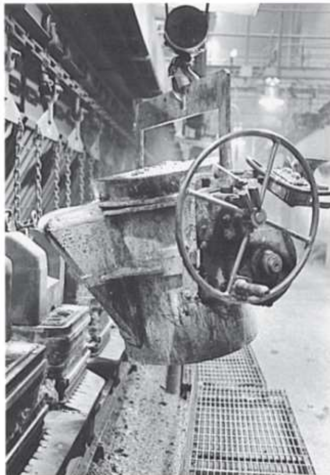
Figure 25-3. This tilting ladle is equipped with a manually operated antitilt level. (Courtesy American Foundrymen's Society, Inc.)
