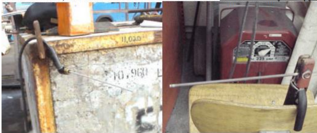
Figure 17 DANGEROUS CONDITION - Unattended Energized Electrode Holder
