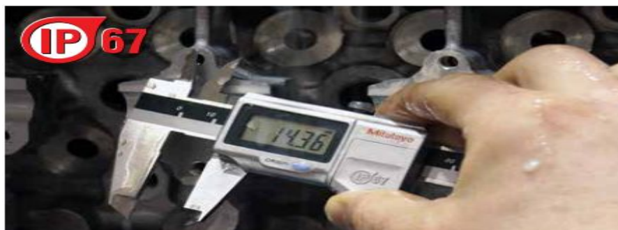
Fig. 2.16. to check the dimension of gear
