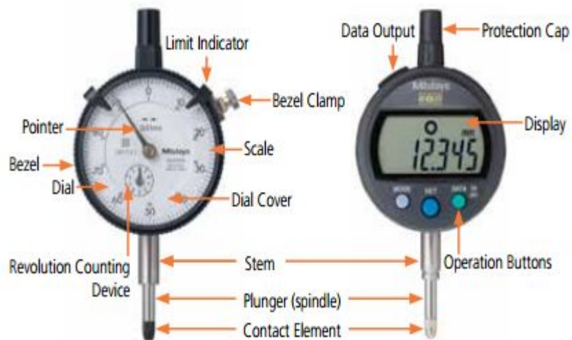
Fig.2.44. parts of indicator
