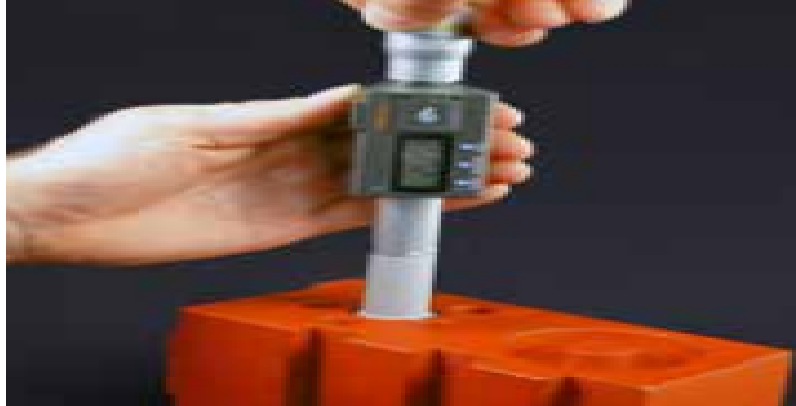
Fig.2.27. Retracting the spindle of a digital 3-point internal micrometer
