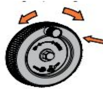
Coarse feed To use coarse feed push the handle in and rotate the whole wheel.
