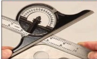
Fig. 3.14. Application a combination square.
