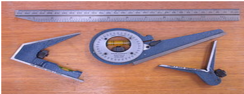
Fig. 1.7. combination square Uses
