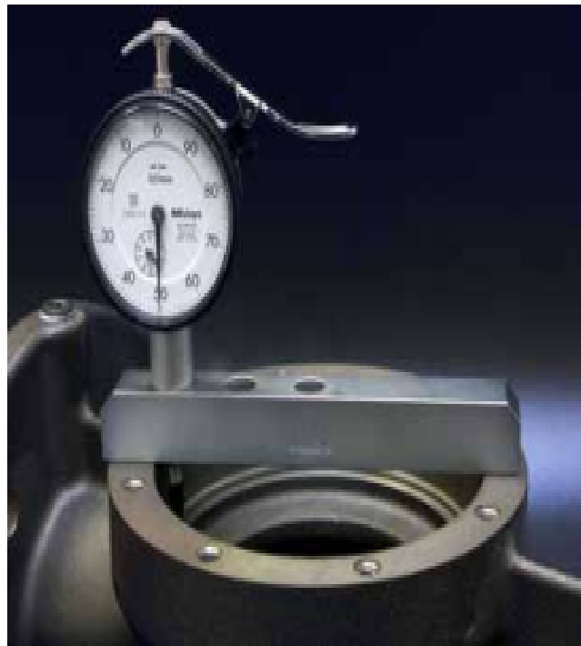
Fig. 2.55. use the gauge in vertical orientation only.
