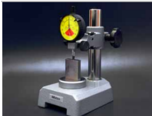
Fig.2.57. Reference point setting with a 50 mm Gauge Block.
