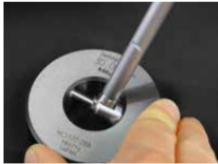
Fig. 2.32. bore gauge into the hole to be measured
