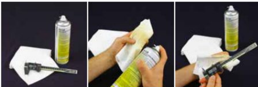
Fig.2.10. apply anti-corrosive coating for rust prevention
