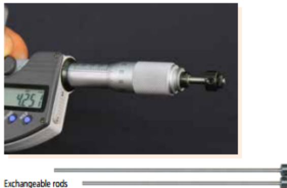
Fig.2.53. contacting surfaces on the rod collar and spindle end.
