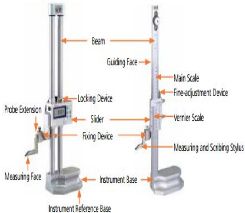
fig 2.39. detail parts of height gauge
