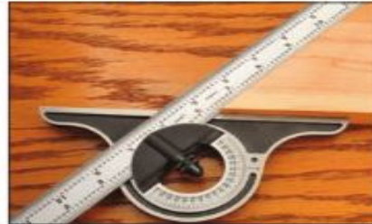
Fig. 3.14. Application a combination square.
