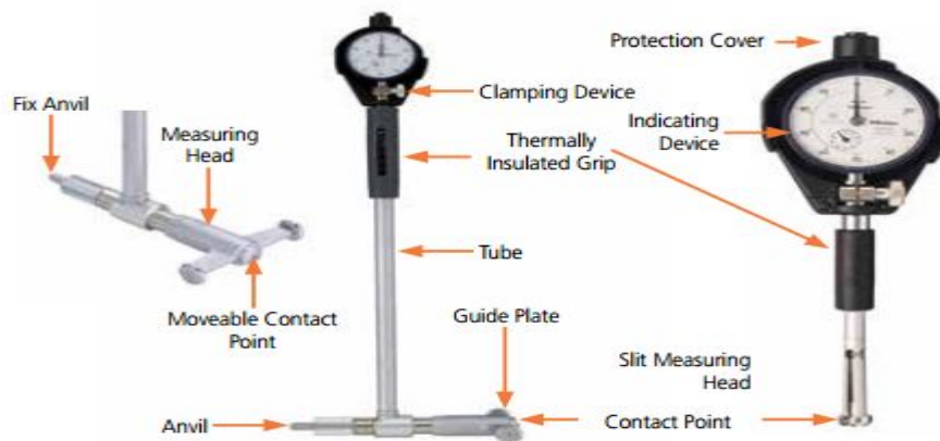
Fig.2.29. 2. parts of -Point Internal Measuring Instruments
