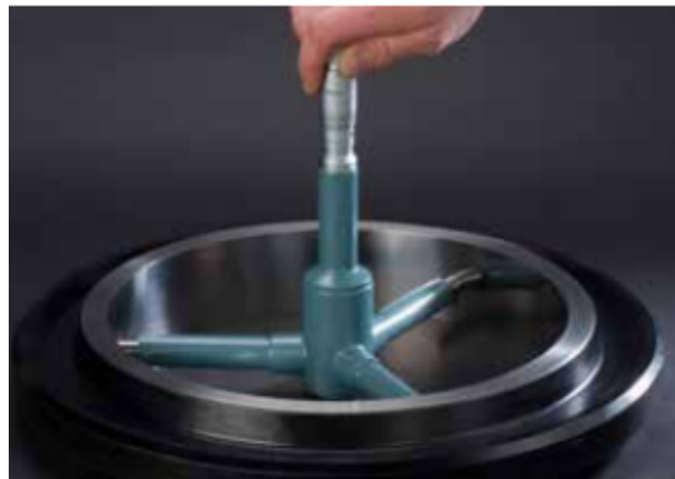
Fig.2.25. calibration of master gauge
