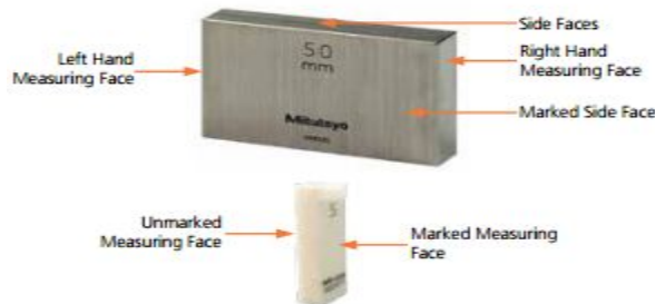
Fig. 2.59. parts of gauge block Before Use
