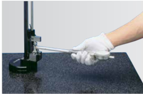
Fig. 2.30. bore gauge checker with gauge blocks
