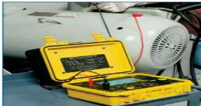
Fig.1.21. Measuring insulation resistance
