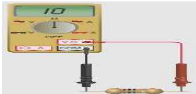
Fig. 2.19. Ohmmeter connected to measure resistance.
