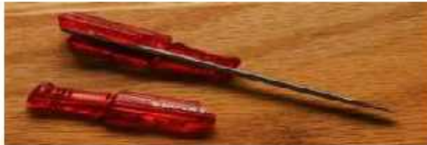
Screw driver with a broken handle
