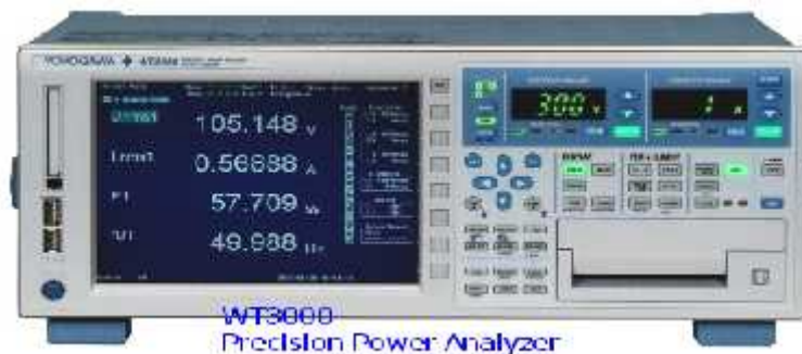
Fig.1.22. precision of power measurement Analyzer
