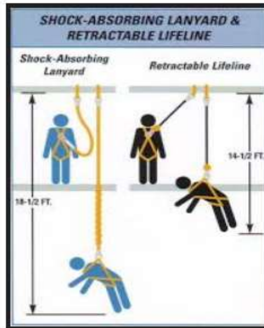
Figure 7: The required length of the lifeline (GIZ, 2016)
