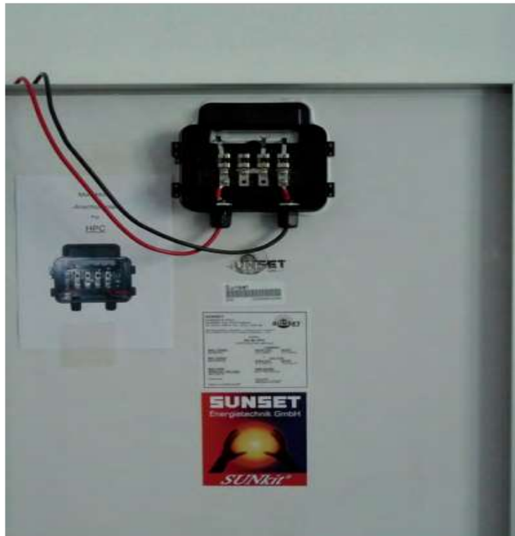
Figure 10: Back of module showing leads from junction box (Hankins, 2010)
