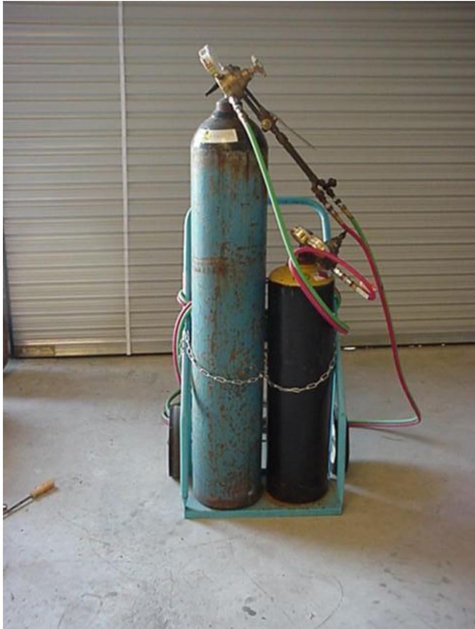
Fig. Assembled oxy acetylene cutting out fit
