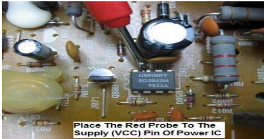
Figure3.20. Placing the RED test probe to the positive pin of the Filter Capacitor.
