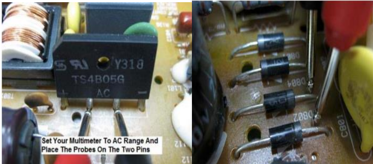
Figure3.18. Placing the test probes to Two AC Pins (a) Single Package and (b) individual Diode.
