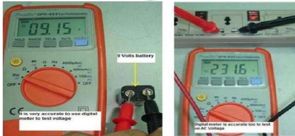
Figure6.5 Measuring the voltage using digital meter.
