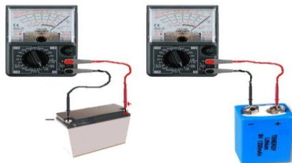
Figure6.9. Caution in measuring resistance
