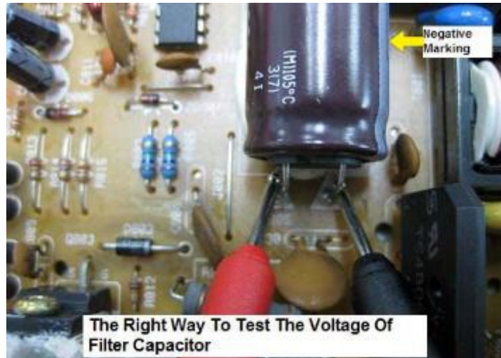
Figure3.19. Testing voltage at the filter capacitor
