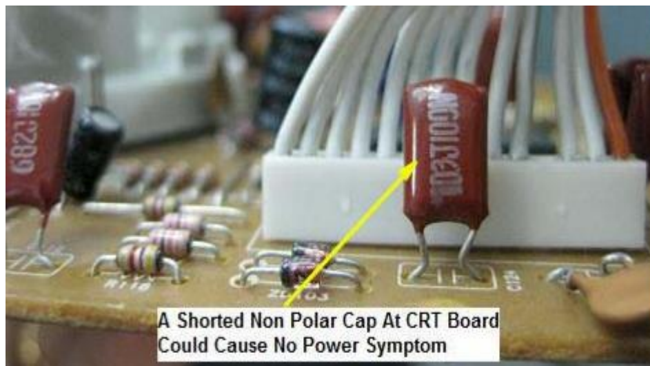
Figure4.1 Shorted Non Polar Capacitor at CRT Board.
