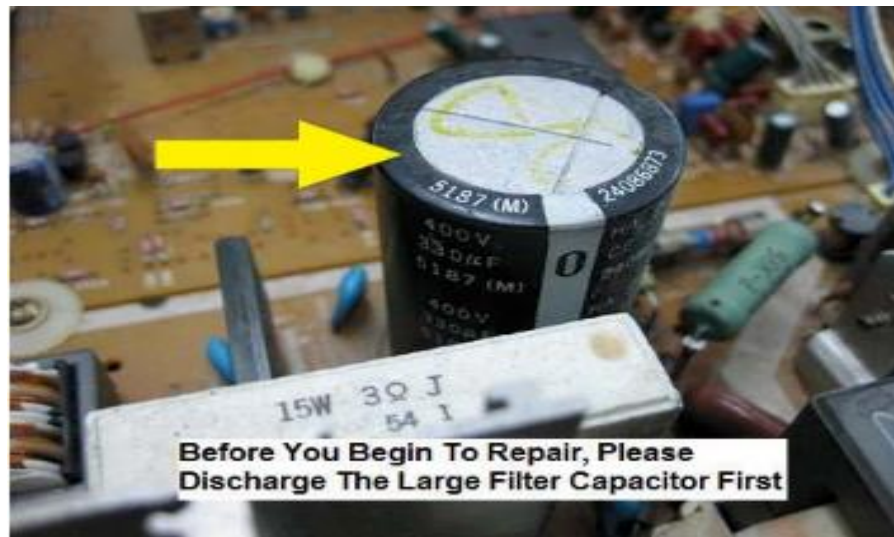
Figure5.1 Discharging the Big Capacitor
