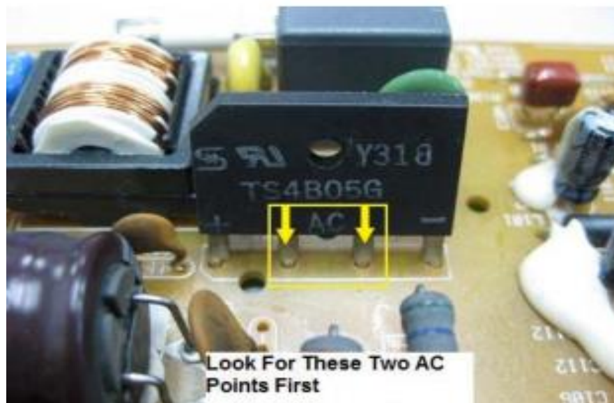
Figure3.17. Two AC Pins of a Bridge Rectifier on a Single Package.
