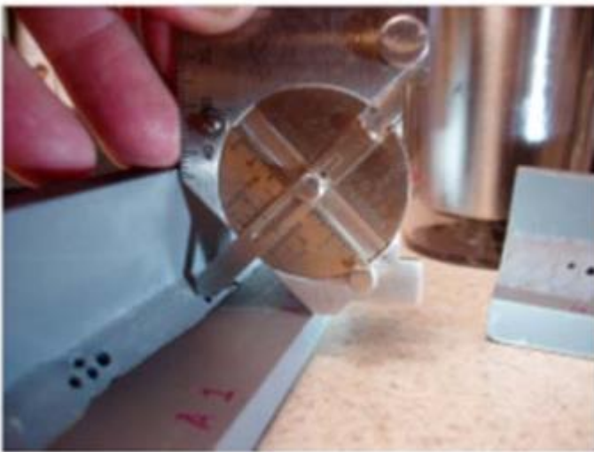
Figure 2.3: Throat measurement with cam gauge
