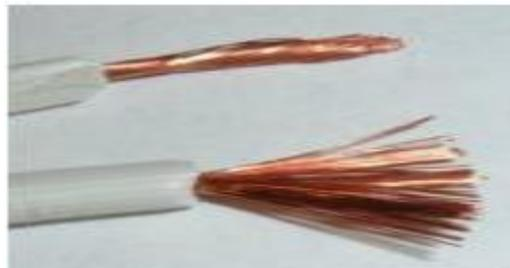
Fig.1.2 stranded conductor
