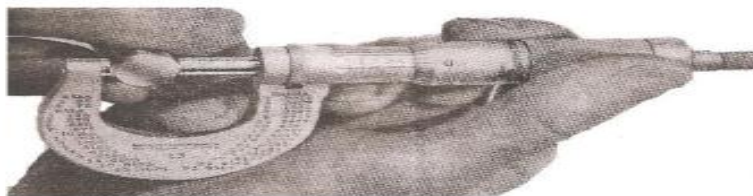
Fig. 3.1 This is how to hold the micrometer correctly when piece is held in the hand.
