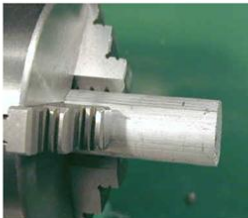
Fig: Facing work on lathe machine
