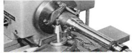
Machining work mounted between centers.
