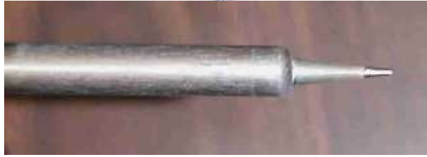
Fig3. A properly cleaned and “wetted” soldering iron tip.
