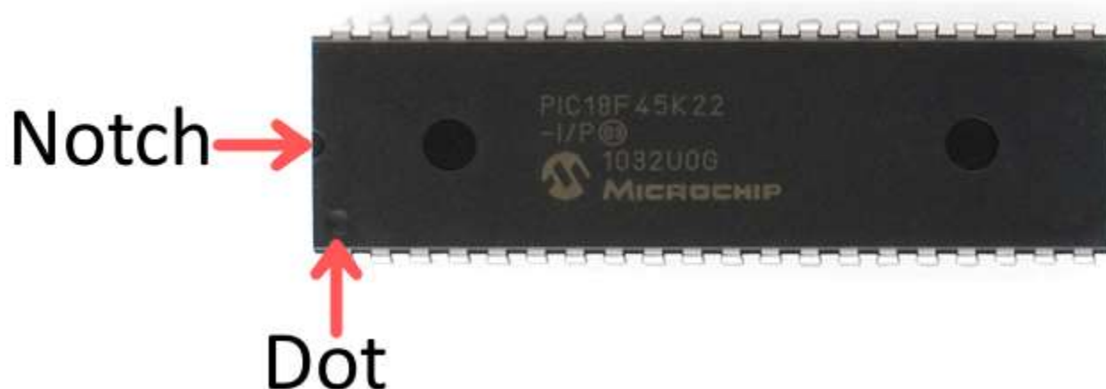
Fig 3.8. Polarity and pin numbering of ICs
