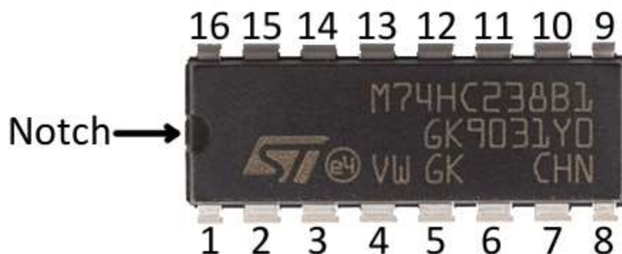
Fig 3.9. Polarity and pin numbering of ICs
