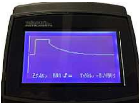
An oscilloscope displaying capacitor discharge
