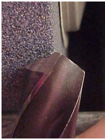
Fig2.10. Line up the end of the web with the corner of the wheel.
