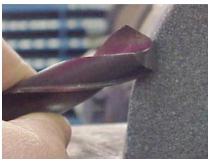
Fig2.9. Holding the drill at a 30- degree angle
