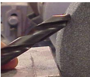
Figure 2.12. The approach angle is steeper when web splitting than it is when web thinning.
