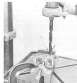
Fig1.2. Tighten the table clamp.
